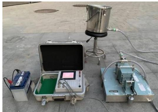
**Figure 1.** Dynamic Friction Tester.
