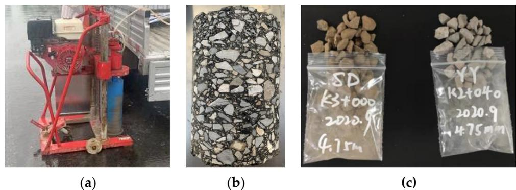
**Figure 2.** Extraction process of coarse aggregates in the core samples from the asphalt pavement. (a) In-situ core-drilling; (b) Drilled core sample; (c) Coarse aggregates extracted in core sample.
