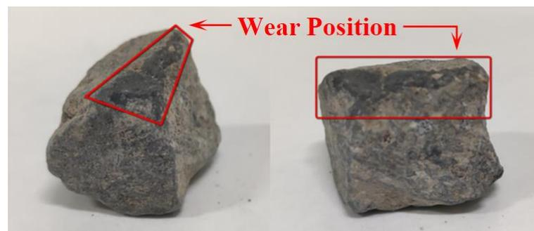
**Figure 6.** Schematic diagram of coarse aggregate wear position.
