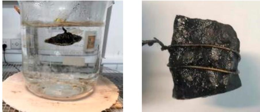
**Figure 1.** A sketch of the Chinese boiling water test.
