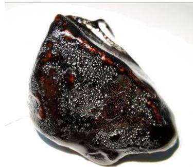
**Figure 3.** The aggregate after boiling water test on a white slab.
