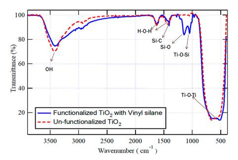
**Figure 2.** FT-IR for both vinyl-functionalized and un-functionalized TiO<sub>2</sub> nanoparticles in the selected wavenumber ranges.
