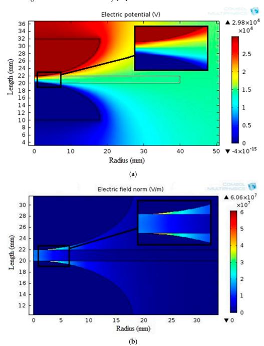
**Figure 10.** Distributions of (**a**) potential and (**b**) electrostatic field around mushroom-to-mushroom electrode for the varnish/0.4 wt.% TiO<sub>2</sub> nanocomposite.
