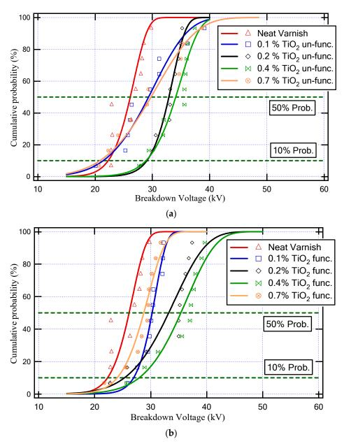
**Figure 8.** Weibull cumulative probability against breakdown voltage for various neat varnish and varnish/ $TiO_2$  nanocomposite samples; (a) unfunctionalized  $TiO_2$  and (b) functionalized  $TiO_2$ .
