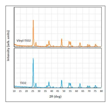
Figure 3. XRD diffractograms of TiO<sub>2</sub> and the functionalized Vinyl TiO<sub>2</sub> nanoparticles.
