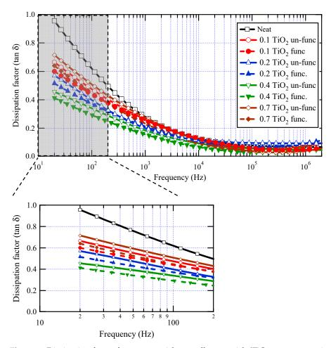
**Figure 7.** Dissipation factor for neat varnish as well as varnish/TiO<sub>2</sub> nanocomposites for various filler contents.
