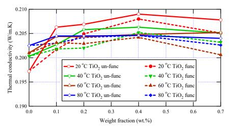
Figure 5. Thermal conductivity analysis for varnish nanocomposites and neat varnish.
