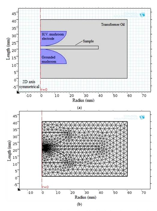
Figure 9. BDS computation via (a) the obtained model and (b) the finite element meshes shape.
