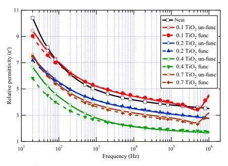
**Figure 6.**  $\varepsilon'$  for neat varnish and varnish/TiO<sub>2</sub> nanocomposites for different loading of nanoparticles.
