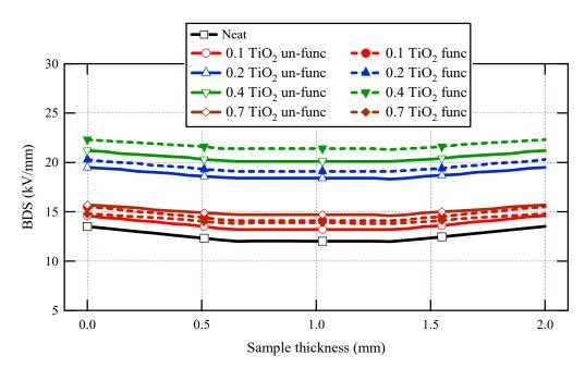
**Figure 11.** AC-Breakdown strength for neat varnish as well as varnish/TiO<sub>2</sub> nanocomposites for various filler contents.
