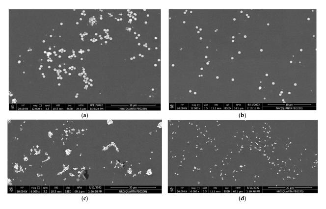
**Figure 4.** FE-SEM micrographs of Varnish/TiO<sub>2</sub> nanocomposites: (**a**,**c**) are for 0.1% un-functionalized TiO<sub>2</sub> at magnifications 12,000× and  $6000\times$ , respectively, and (**b**,**d**) are for 0.1% functionalized TiO<sub>2</sub> at 12,000× and  $6000\times$ , respectively.
