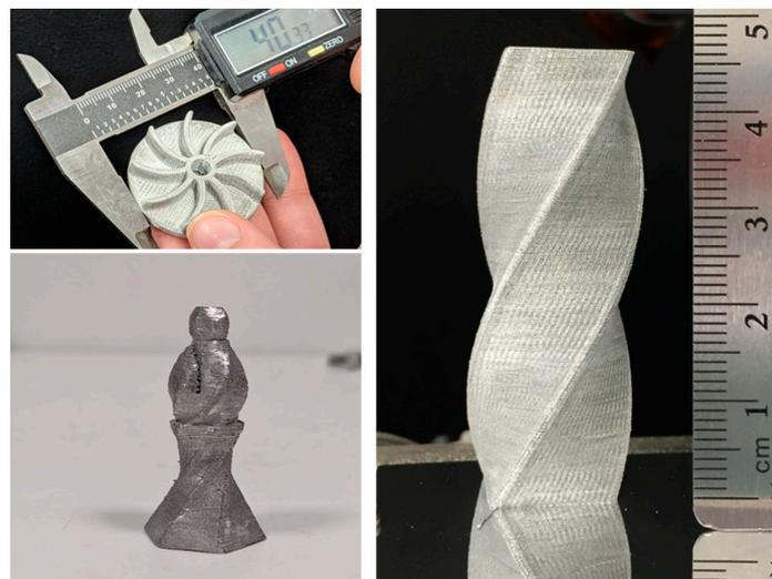
**Figure 2.** Aluminum 6061 alloy objects fabricated using the RAD process.
