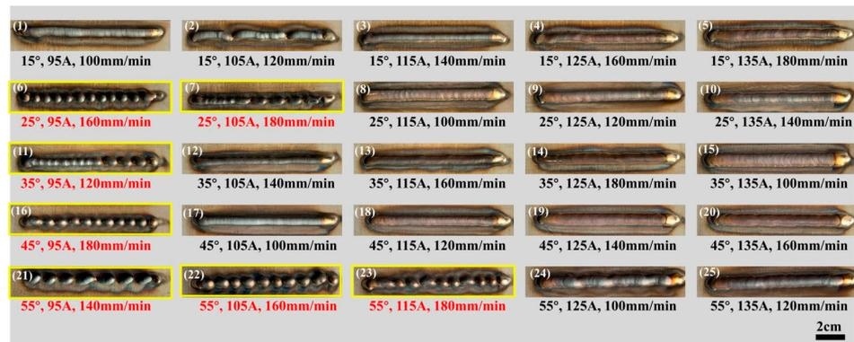
Figure 3. CCD-based design for single-pass, single-layer weld testing.
