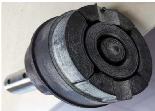
**Figure 11.** An example of a core made using 3D printing is shown in figure.
