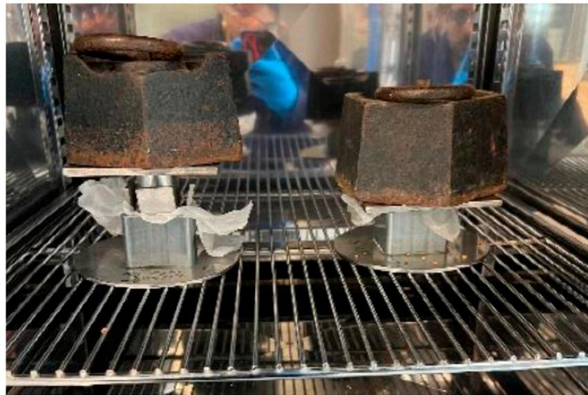
**Figure 2.** Sample mould containing compressed binder/cork mixture within curing oven.
