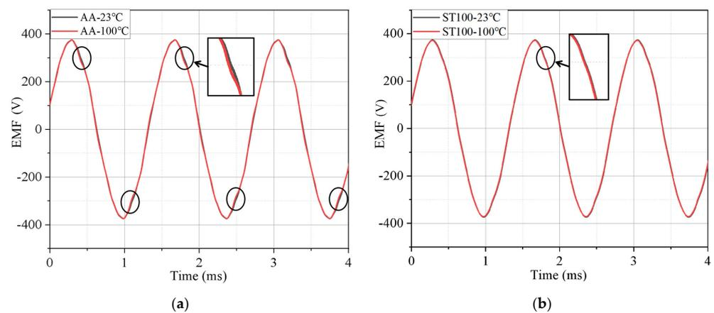
**Figure 15.** Back EMFs of AA and ST100 motors at different temperatures: (a) AA; and (b) ST100.
