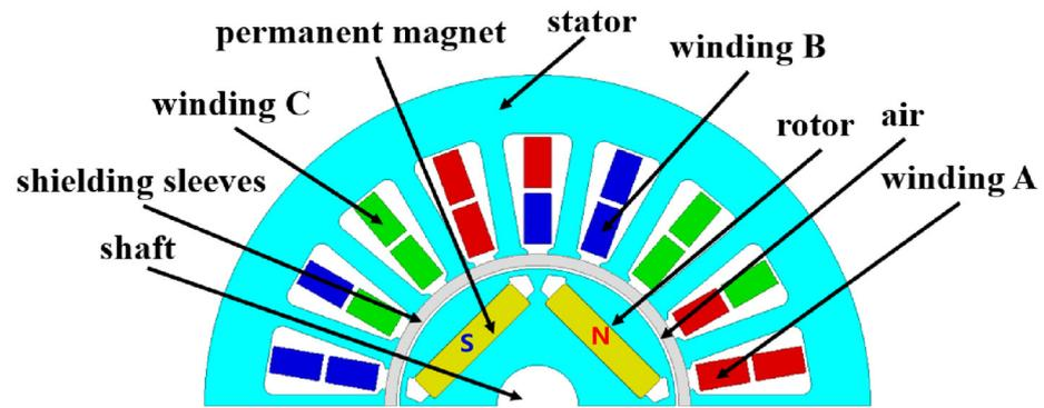
**Figure 11.** Finite element model of permanent magnet synchronous motor.
