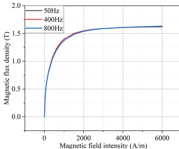
**Figure 5.** Magnetization characteristics of AA at different frequencies (temperature = 23 °C).
