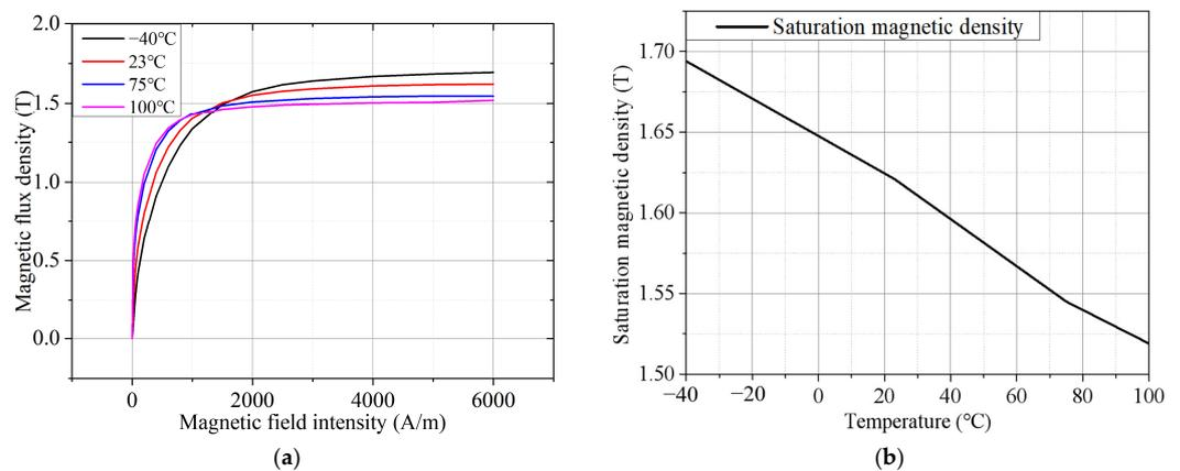
**Figure 4.** Magnetization characteristics of AA at different temperatures (frequency = 50 Hz): (a) B–H curve; and (b) saturation flux density of AA at different temperatures.
