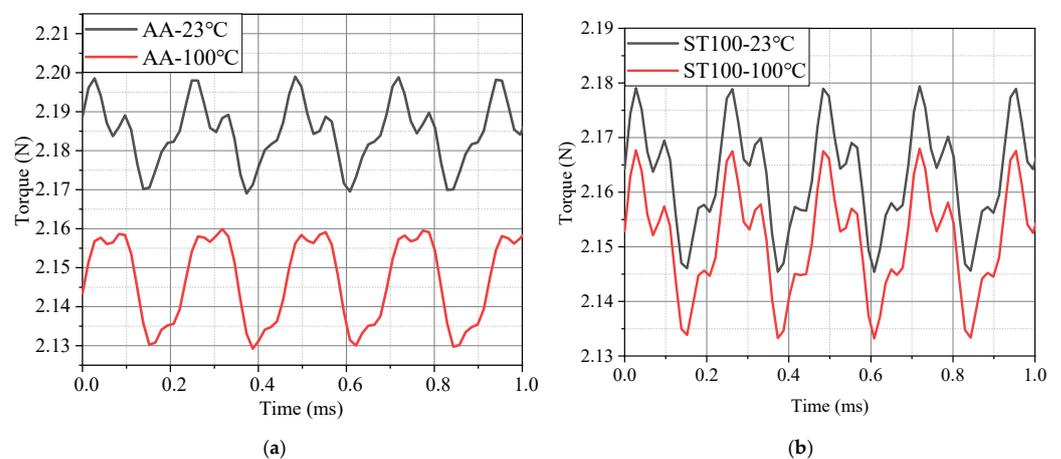
**Figure 16.** Torques of AA and ST100 motors at different temperatures: (a) AA; and (b) ST100.
