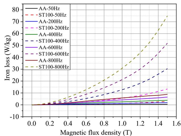
**Figure 8.** Iron loss of AA and ST100 at different test frequencies (temperature = 23 °C).
