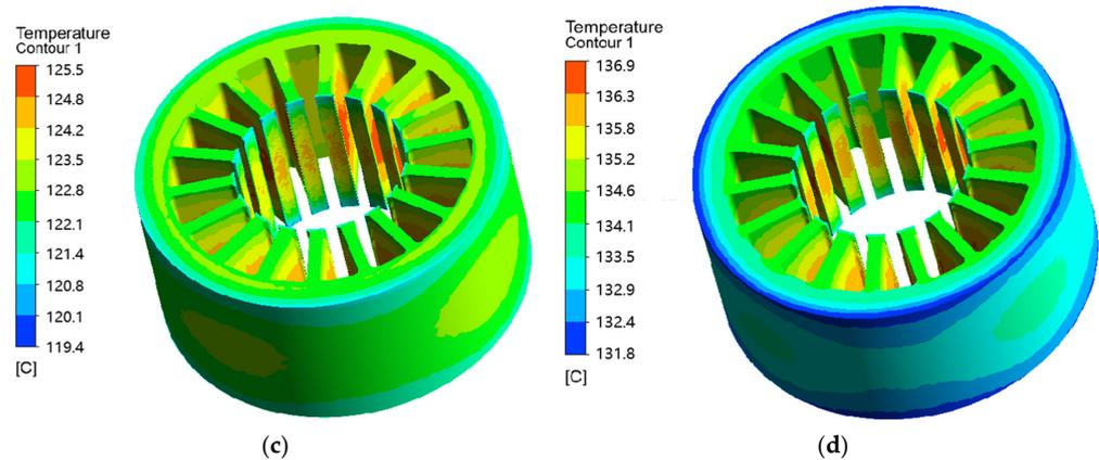
**Figure 12.** Temperature rise cloud image of AA and ST100 motors: (a) AA-no iteration; (b) AA-iteration; (c) ST100-no iteration; and (d) ST100-iteration.
