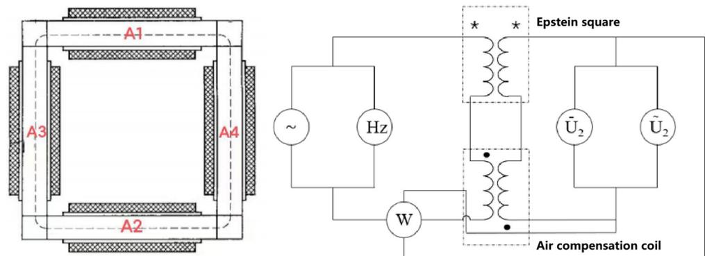
**Figure 2.** The principle of Epstein's square circle method.
