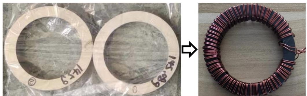
**Figure 3.** Test samples of the magnetic properties of AA and ST100.
