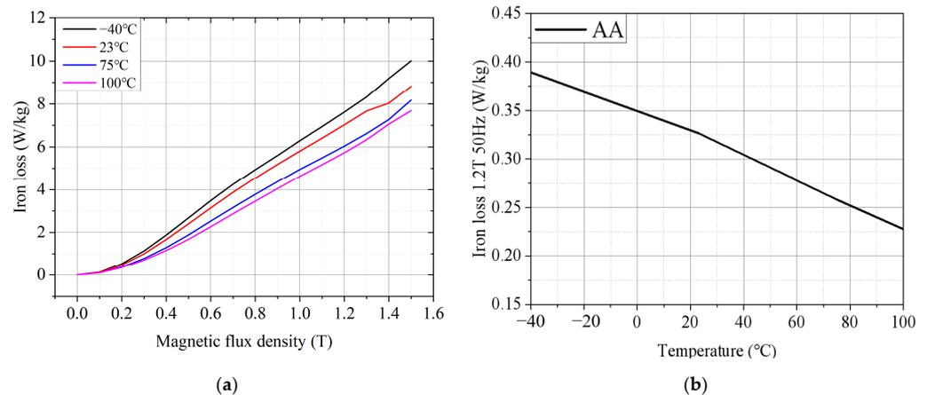
**Figure 6.** Iron loss characteristics of AA at different temperatures: (a) B–P curve (frequency = 800 Hz); and (b) iron loss of AA at different temperatures (frequency = 50 Hz, magnetic flux density = 1.2 T).
