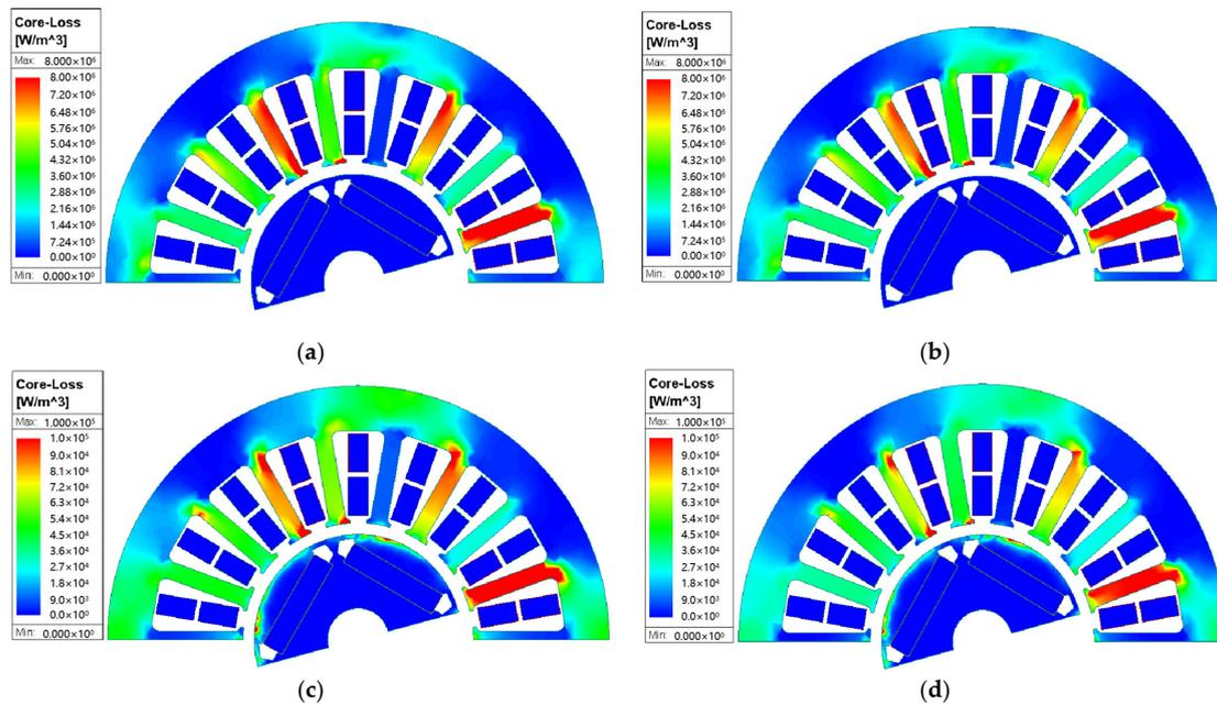
**Figure 14.** Iron loss distribution of AA and ST100 motors at different temperatures: (a) ST100-23 °C; (b) ST100-100 °C; (c) AA-23 °C; and (d) AA-100 °C.
