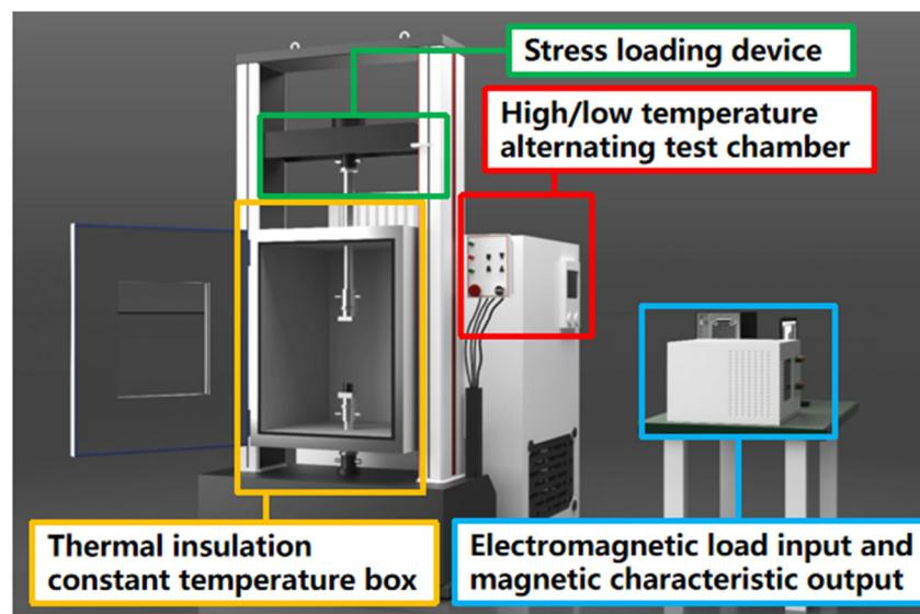
**Figure 1.** Multi-physical field testing equipment for magnetic properties of soft magnetic materials.
