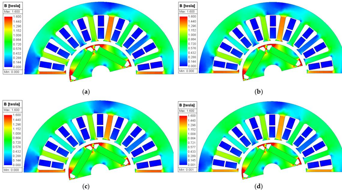
**Figure 13.** Magnetic flux density distribution of AA and ST100 motors at different temperatures: (a) ST100-23 °C; (b) ST100-100 °C; (c) AA-23 °C; and (d) AA-100 °C.
