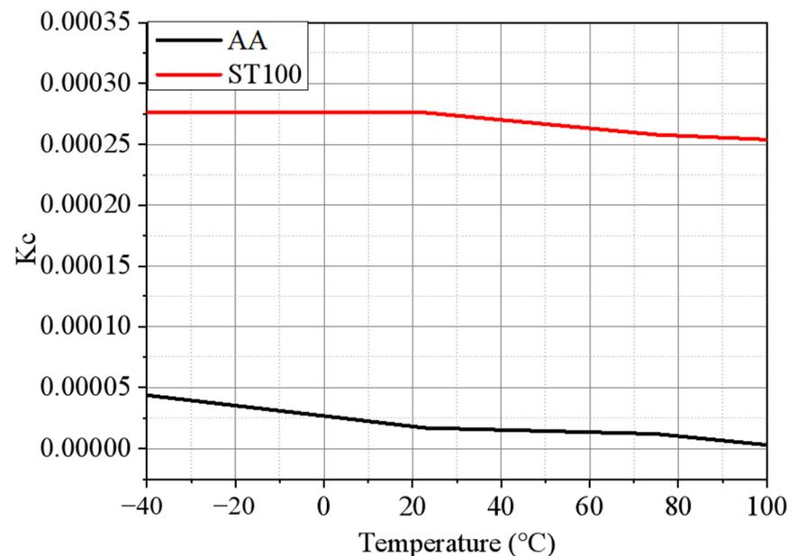
Figure 10. Eddy current loss coefficient of AA and ST100 at different temperatures (frequency = 50 Hz).
