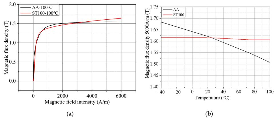
**Figure 7.** Magnetization properties of AA and ST100 (frequency = 50 Hz): (a) B–H curve; and (b) magnetic flux density of AA and ST100 at different temperatures (magnetic field intensity = 5000 A/m).
