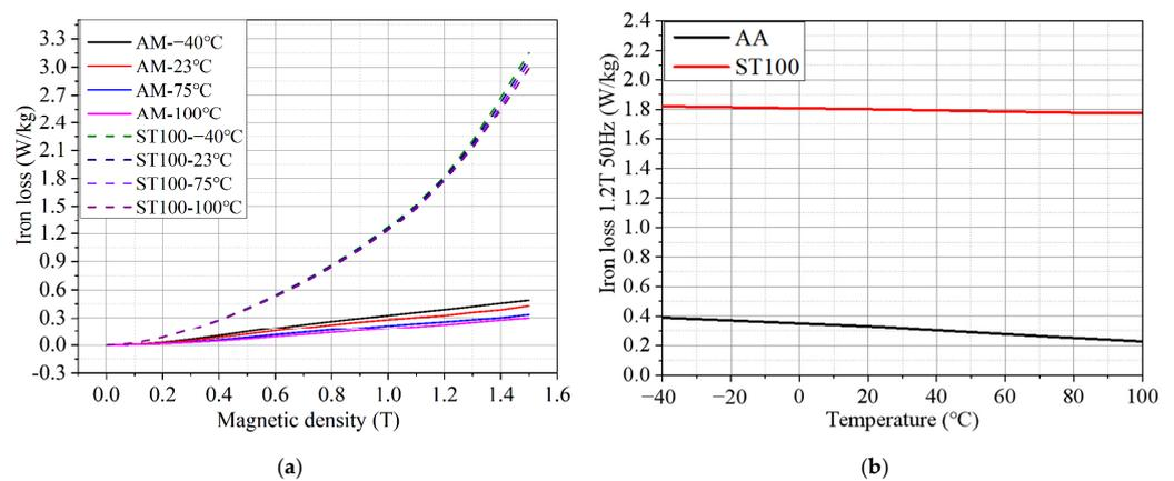
**Figure 9.** Iron loss of AA and ST100 at different temperatures (frequency =  $50\text{ Hz}$ ): (a) B–P curve; and (b) iron loss of AA and ST100 at different temperatures (magnetic flux density =  $1.2\text{ T}$ ).
