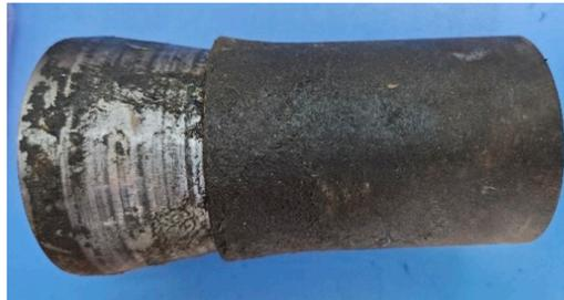
**Figure 2.** Expansion cone and pipe.
