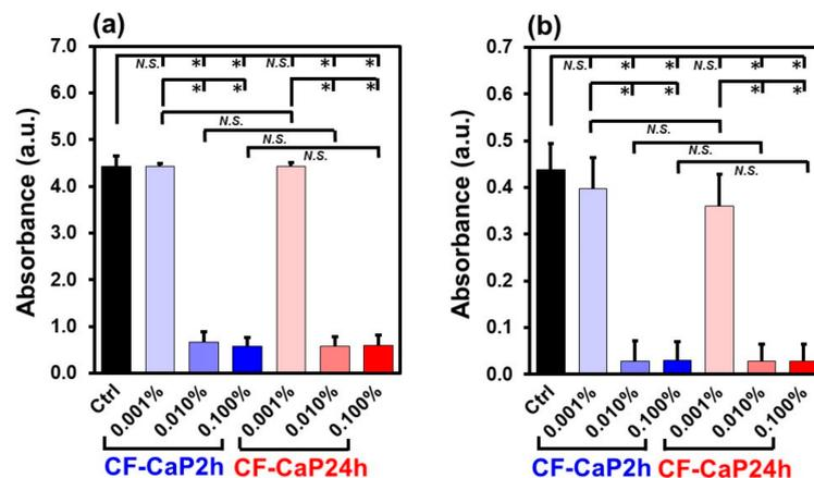
**Figure 10.** (a) Relative amounts of biofilms (absorbance at 595 nm) and (b) relative metabolic activity of the bacterial (*S. mutans*) biofilm (absorbance at 450 nm), after incubation of *S. mutans* in the presence of CF-CaP2h and CF-CaP24h at various doses: 0 (Ctrl), 0.001, 0.01, and 0.1 w/v% (n = 6, average + SD, \* p < 0.05, N.S.: not significant).
