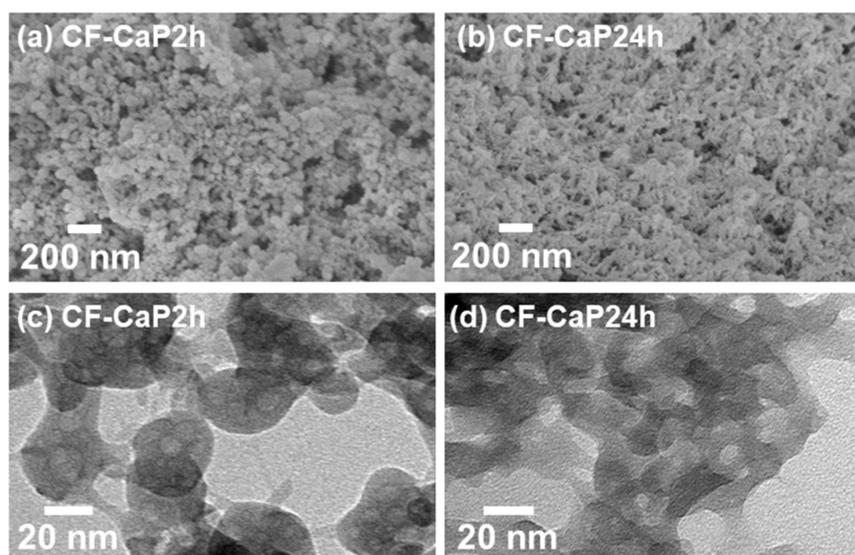
**Figure 3.** (a,b) FESEM and (c,d) TEM images of (a,c) CF-CaP2h and (b,d) CF-CaP24h.
