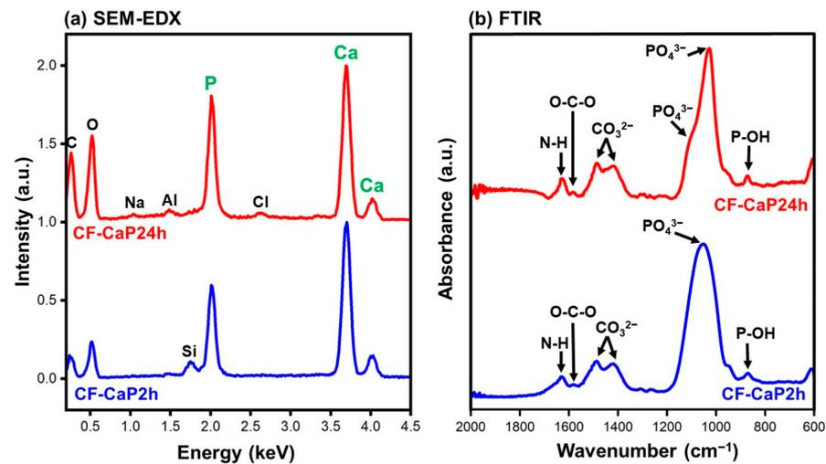
**Figure 4.** (a) SEM-EDX and (b) FTIR spectra of CF-CaP2h and CF-CaP24h. The peaks of Al and Si in (a) are from the sample holders.
