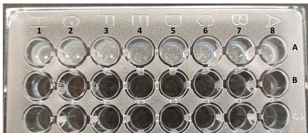
Figure 4. The plastic container with the iodine-based agents: A—NaDITMB, B—Omnipaque. The volumes of solutions in cylindrical cavities 1 to 3 were 0.2 mL, while those in cavities 4 to 8 were 0.1 mL each, maintaining a constant iodine concentration.
