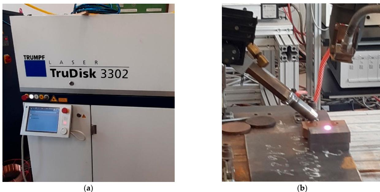
**Figure 2.** The disc laser used in tests: (a) control panel, (b) remelting process of sample surface.
