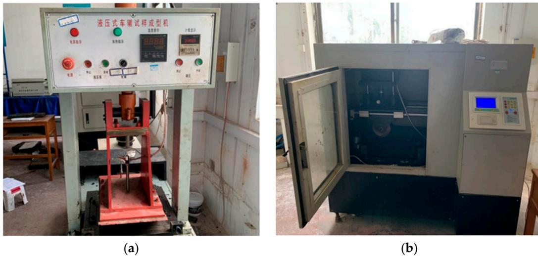
**Figure 5.** The rutting test equipment: (a) rutting sample forming machine, (b) wheel-track test machine.
