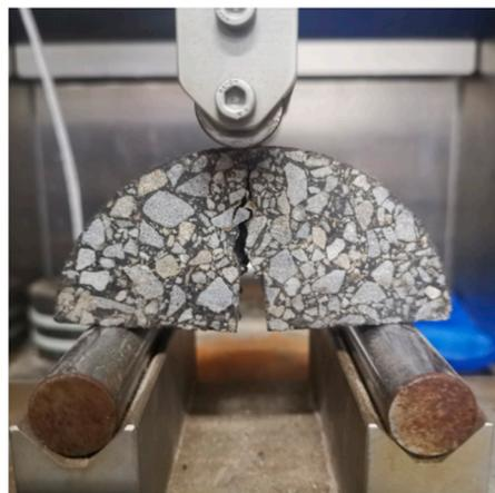
**Figure 6.** Semi-circular specimen test set.
