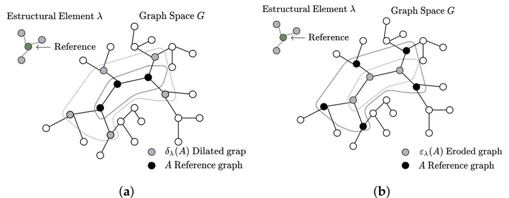
Figure 1. Morphological basic operators: (a) dilation operator and (b) erosion operator.
