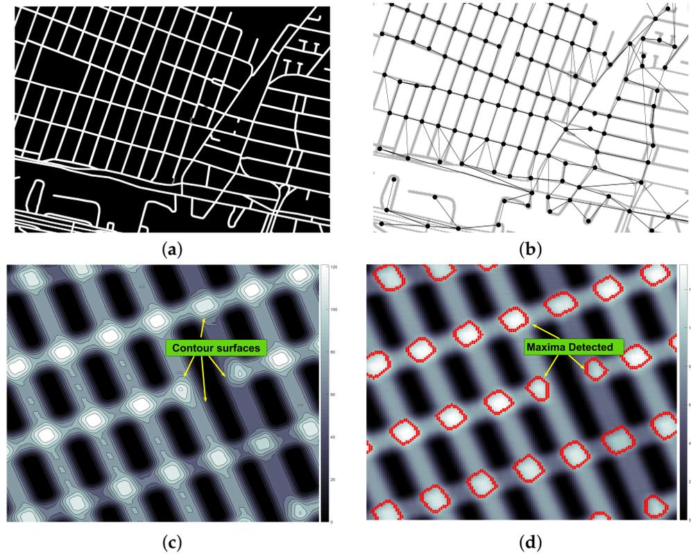
**Figure 5.** Map encoding process: (a) geographical binary map layer; (b) built graph connection; (c) computation of distance transformation; and (d) detection of maximum zones.
