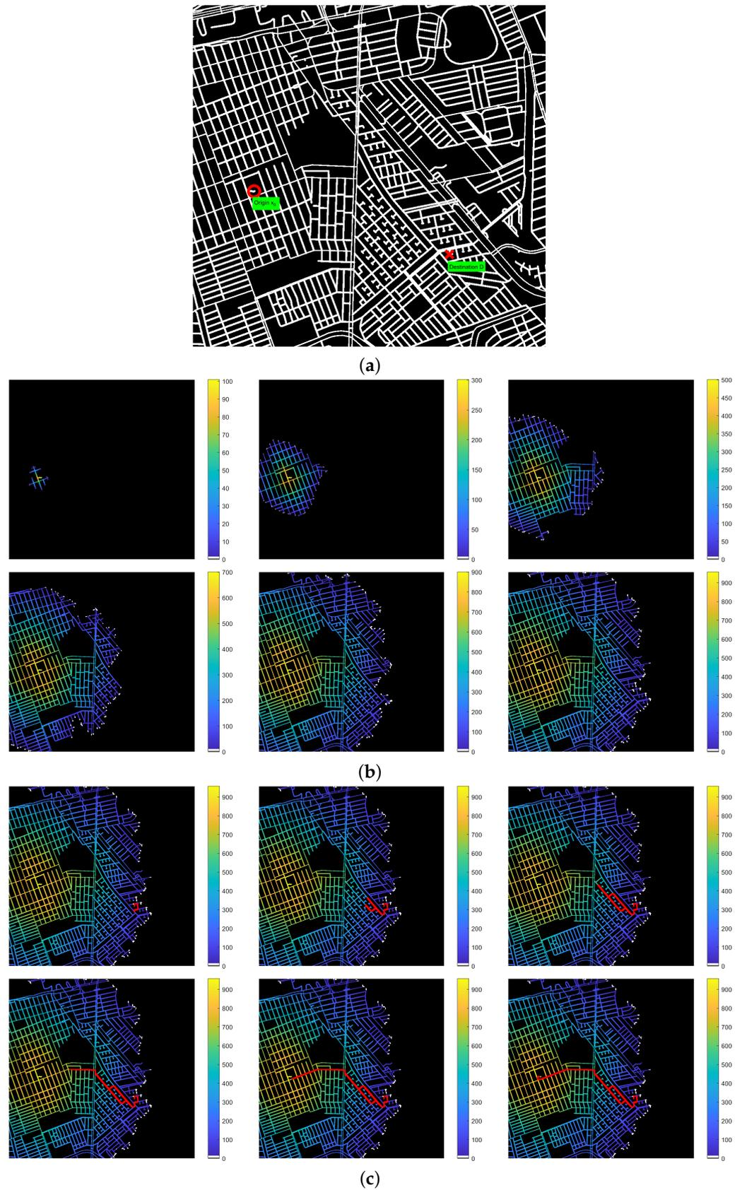
**Figure 3.** Example of searching algorithm with (a) avenue scenario with node origin and destination; (b) frequency with which dilation is applied; and (c) dilations required to reach the goal.
