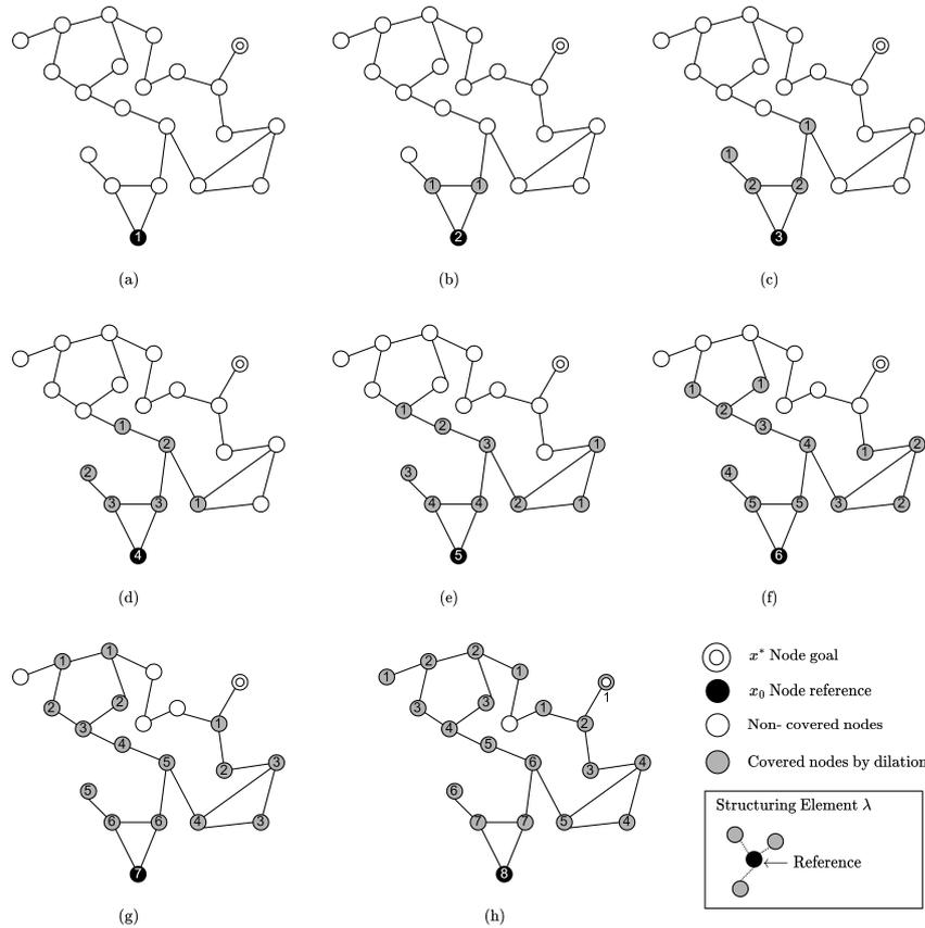
**Figure 2.** Covering dilation operator and the frequency with which each node is dilated.
