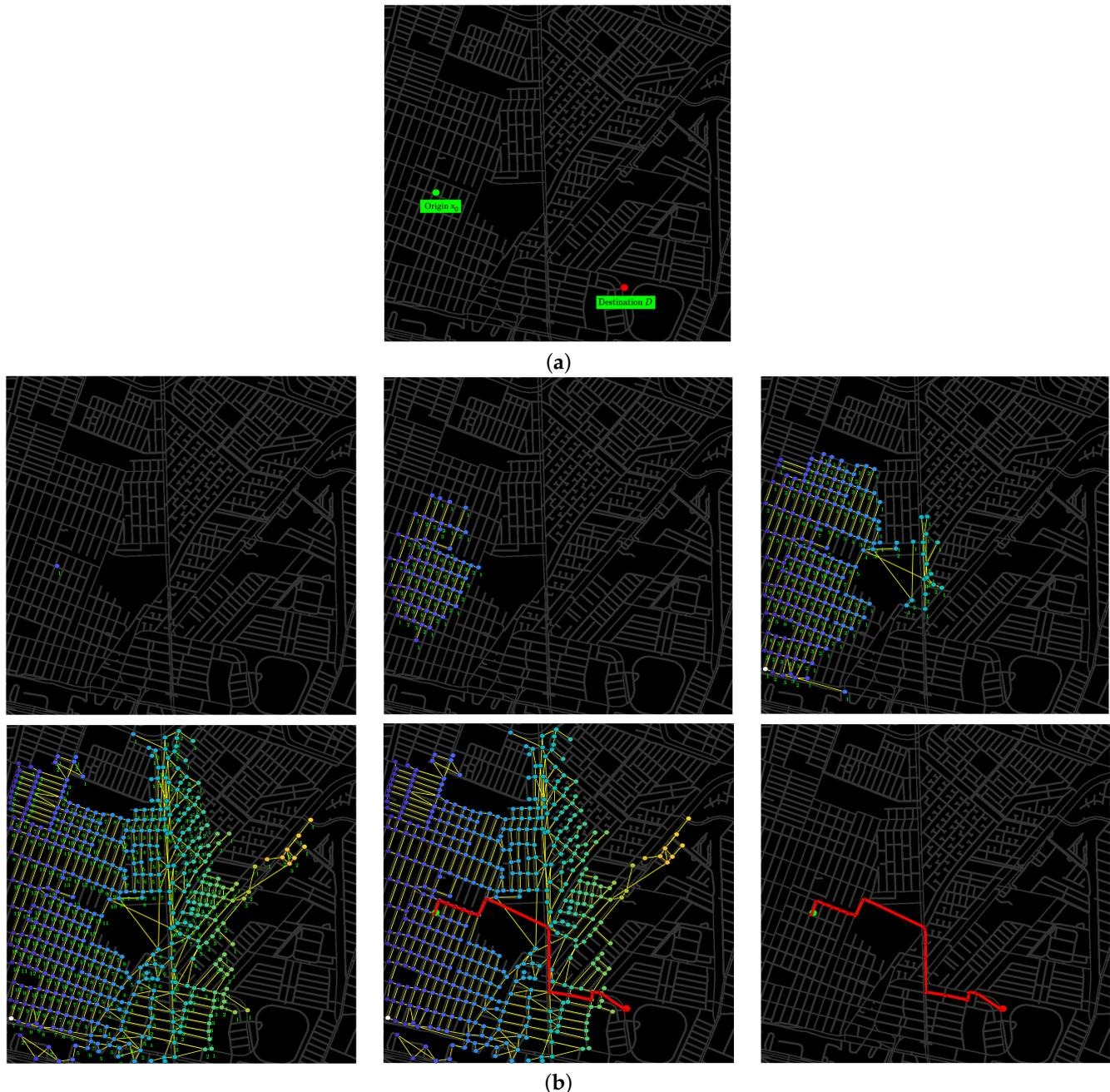
**Figure 6.** Example of the searching algorithm in a graph space with (a) an avenue scenario, including the origin and destination nodes, and (b) the frequency with which dilation is applied and the computation of the best path trajectory.
