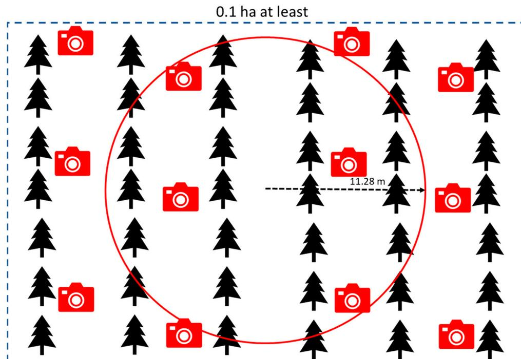
**Figure 6.** Scheme of measuring with the Trestima application.
