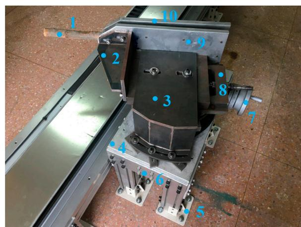
**Figure 3.** The branch clamping device: (1) poplar branches; (2) fixture holder; (3) fixture support frame; (4) connecting plate; (5) foundation base; (6) frame; (7) division plate; (8) dovetail sliding table; (9) internal fixture; (10) external fixture.
