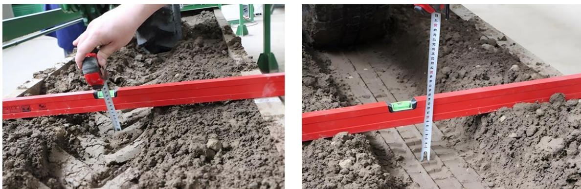
**Figure 11.** Rut depth measuring.
