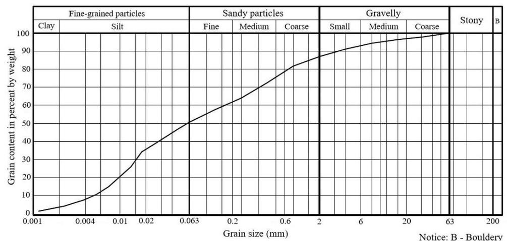
Figure 4. Soil grain size curve.
