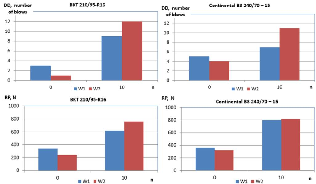
**Figure 20.** Dynamic density ( $DD$ ) and resistance of penetration ( $RP$ ) dependence on the pass number ( $n$ ) at different levels of support surface humidity ( $W1, W2$ ).
