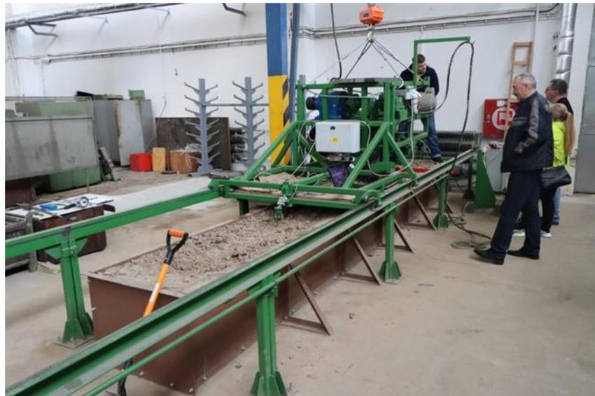
**Figure 5.** Research stand “soil channel”.
