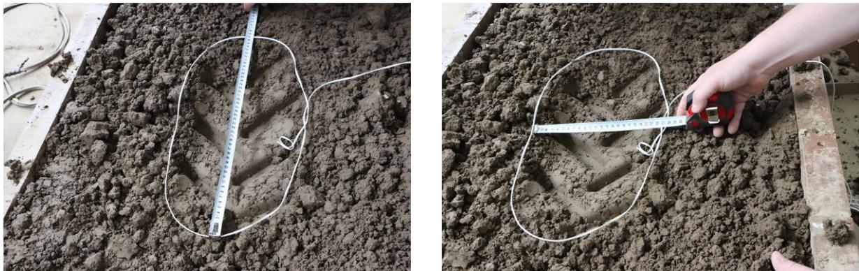
**Figure 8.** Setting the dimensions of the wheel track on the supporting surface of the ground.
