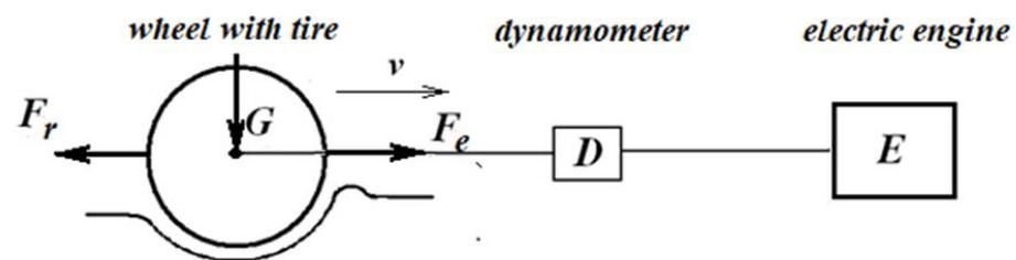
**Figure 3.** Scheme of the experiment on the laboratory stand.
