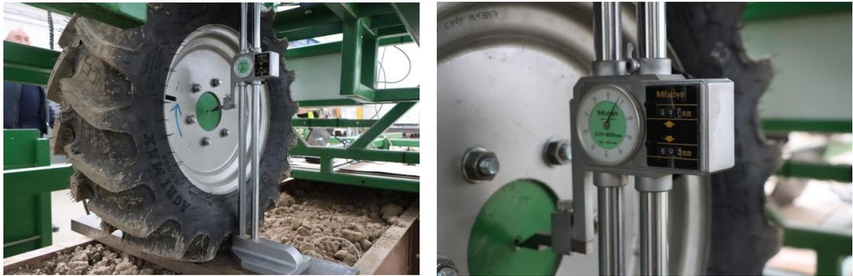
**Figure 7.** Measurement of the static wheel radius using an electronic ruler.
