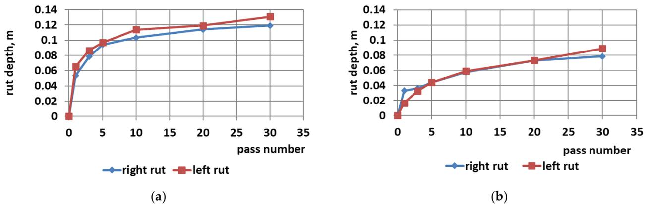
Figure 14. Dependencies of rut depth on the forwarder number of passes: (a) area without branches; (b) area is reinforced with branches.
