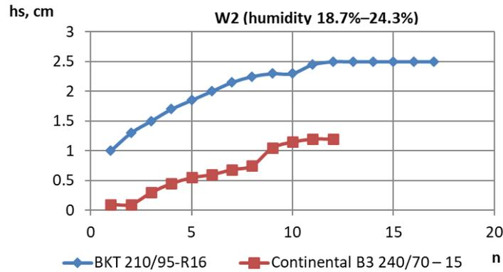
Figure 16. Height of the lateral squeeze dependence ( $h_s$ ) on the pass number ( $n$ ).
