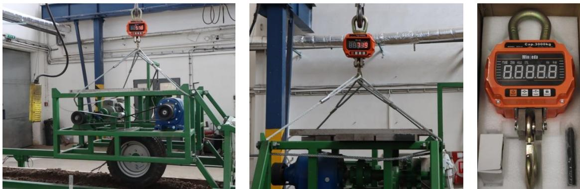
**Figure 9.** Measuring the mass of the carriage with a wheel.
