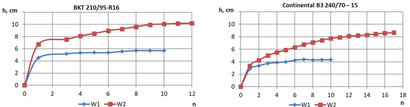
Figure 15. Rut depth dependence ( $h$ ) on the pass number ( $n$ ) at different levels of support surface humidity.
