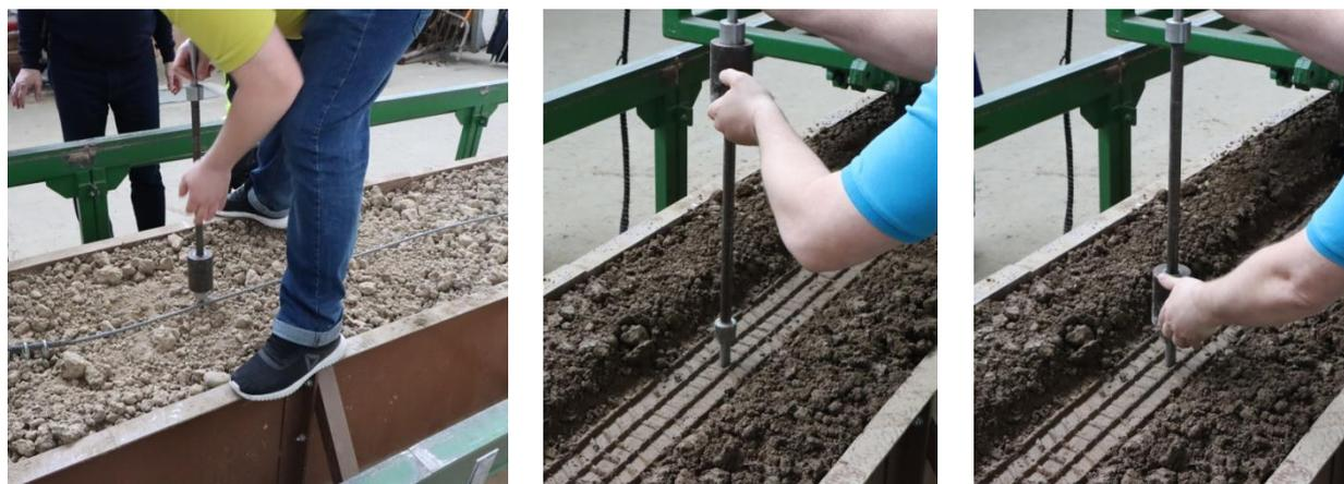
**Figure 12.** Determining the dynamic density of the soil using the DORNII device.
