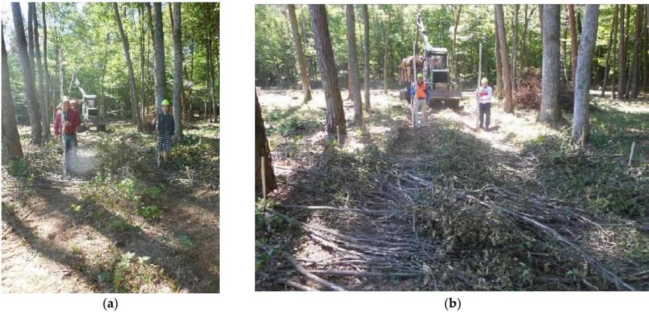
**Figure 2.** Photo fixation of polygon studies. Track depth measurement after 3 passes (a) and after 10 passes (b).
