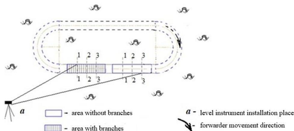
**Figure 1.** Scheme of the landfill for rut formation parameter field studies.
