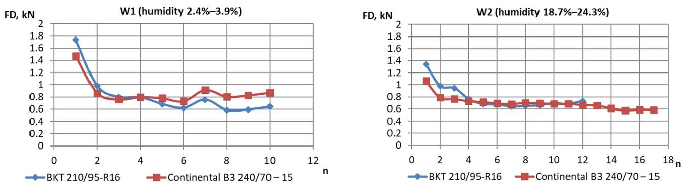
Figure 18. Traction force dependence ( $FD$ ) on the pass number ( $n$ ) at different levels of support surface humidity ( $W_1$ ,  $W_2$ ).
