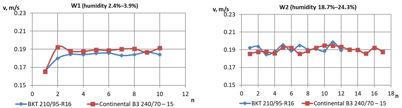
**Figure 19.** Wheel movement speed dependence ( $v$ ) on the pass number of ( $n$ ) at different levels of support surface humidity ( $W1, W2$ ).
