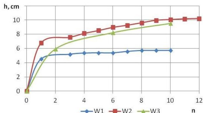
**Figure 21.** Comparison of rutting processes in field and laboratory conditions; W3—field measurements (Figure 14. Area without branches, right track).
