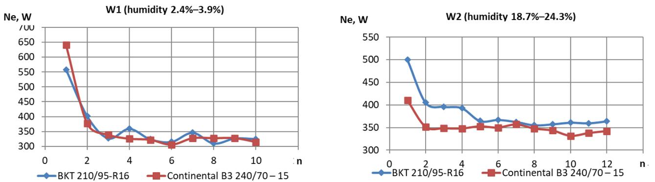
Figure 17. Electric drive power dependence ( $N_e$ ) on the pass number ( $n$ ) at different levels of support surface humidity ( $W_1$ ,  $W_2$ ).
