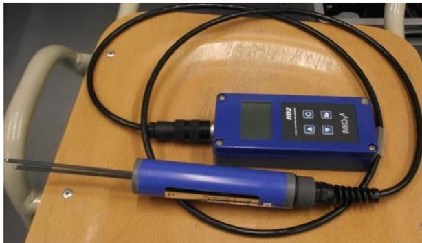
**Figure 10.** Electronic hygrometer Imko HD2 with sensor Trime PICO 64/32.
