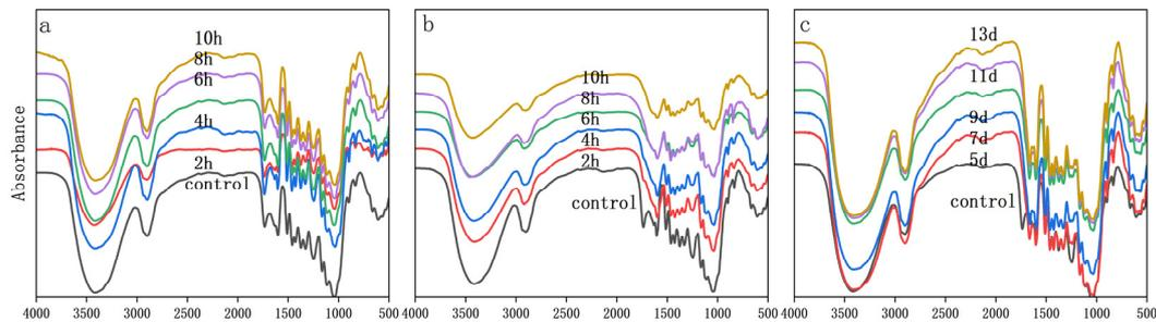
**Figure 8.** Infrared spectra diffraction of bamboo strips for different treatment methods: (a) water boiling, (b) 15% NaOH, and (c) 25%  $\text{NH}_3$  treatment.
