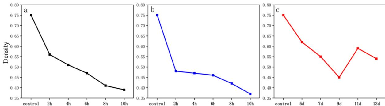
**Figure 4.** Density changes of bamboo strips for different treatments: (a) water boiling, (b) 15% NaOH, and (c) 25% NH<sub>3</sub>.
