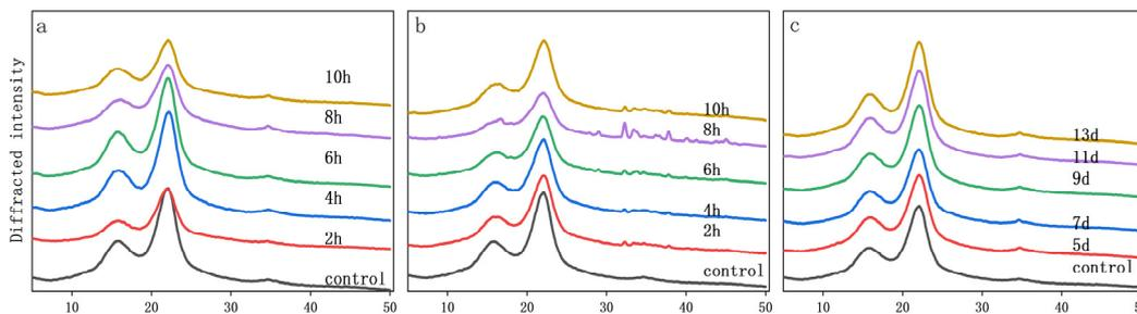
**Figure 7.** X-ray diffraction of bamboo strips for different treatment methods: (a) water boiling, (b) 15% NaOH, and (c) 25% NH<sub>3</sub> treatment.
