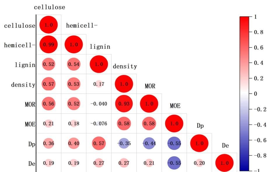
**Figure 10.** Correlation diagram of mechanical and physical properties.
