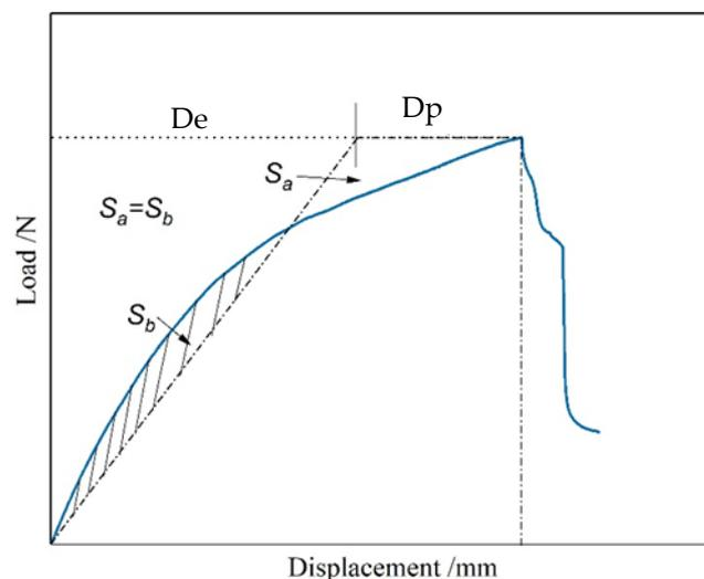
**Figure 2.** Testing method for  $D_e$  and  $D_p$ .
