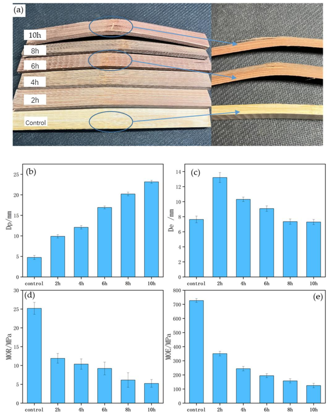
**Figure 3.** Mechanical and physical properties of bamboo strips using water boiling: (a) color and failure status, (b) plastic displacement (Dp), (c) elastic displacement (De), (d) bending strength (MOR), and (e) modulus of elasticity (MOE).
