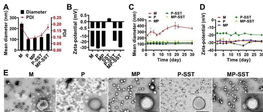
**Figure 2.** Characterization of nanoparticles. (A) The mean diameters and (B) zeta potentials of different nanoparticles and their long-term stabilities of (C) diameters and (D) zeta potentials (mean  $\pm$  SD,  $n = 3$ ). (E) The TEM images showed the morphology of nanoparticles (scale bar = 100 nm in bottom-right magnified images).
