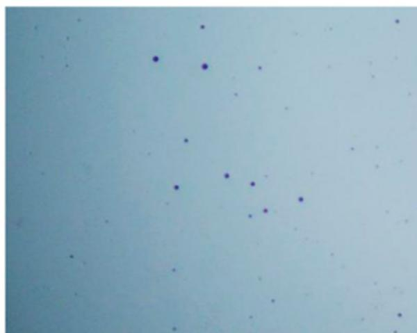
Figure 17. Emulsion No. 1 microscopic image magnified 100 times.
