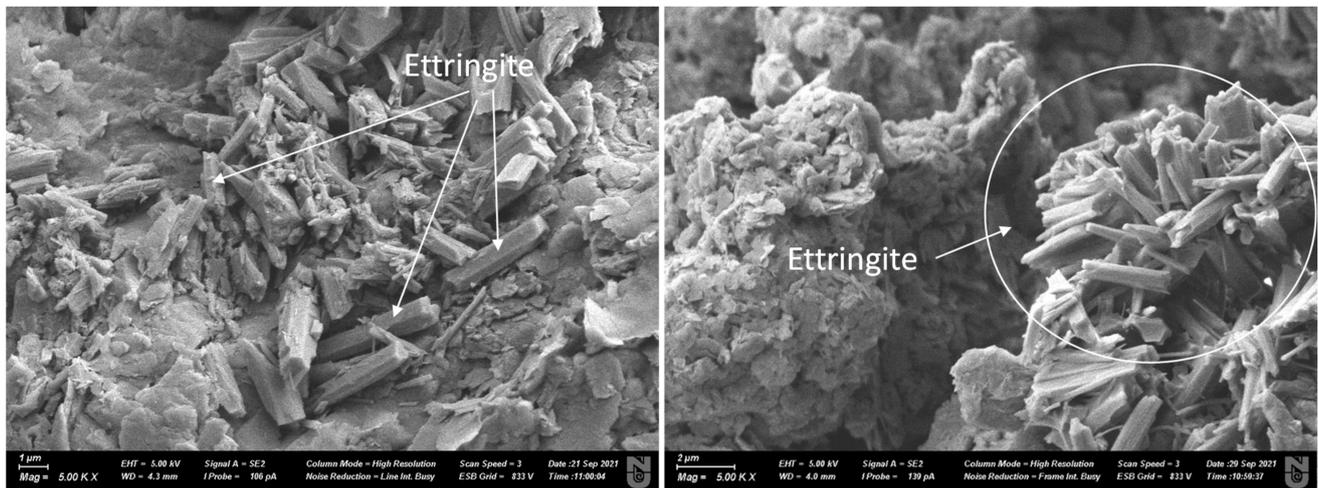
Figure 11. SEM images of soil samples treated with 7% CSA cement cured 14 days at 0 F-T.
