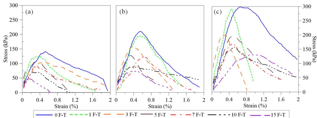
**Figure 5.** Stress-strain response of 14-day cured soil samples treated with CSA cement for all freeze–thaw cycles: (a) 3%; (b) 5%; and (c) 7%.
