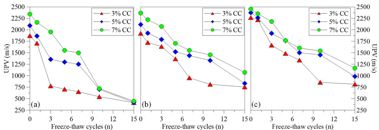
Figure 4. UPV test results: (a) 3-day curing, (b) 7-day curing, and (c) 14-day curing.
