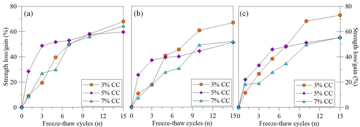
**Figure 9.** Strength loss/gain: (a) 3-day curing; (b) 7-day curing; and (c) 14-day curing.
