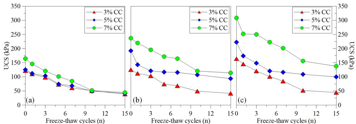
**Figure 6.** UCS test results: (a) 3-day curing; (b) 7-day curing; and (c) 14-day curing.
