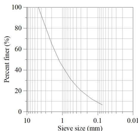
**Figure 2.** Particle size distribution curve for the sand used in this study.
