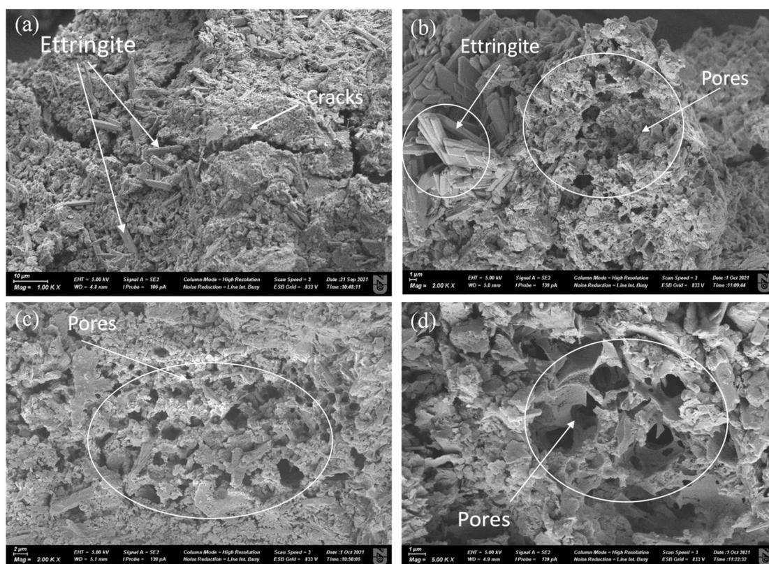
**Figure 12.** SEM images taken after F-T cycles: (a) 1 F-T; (b) 3 F-T; (c) 5 F-T; and (d) 10 F-T.
