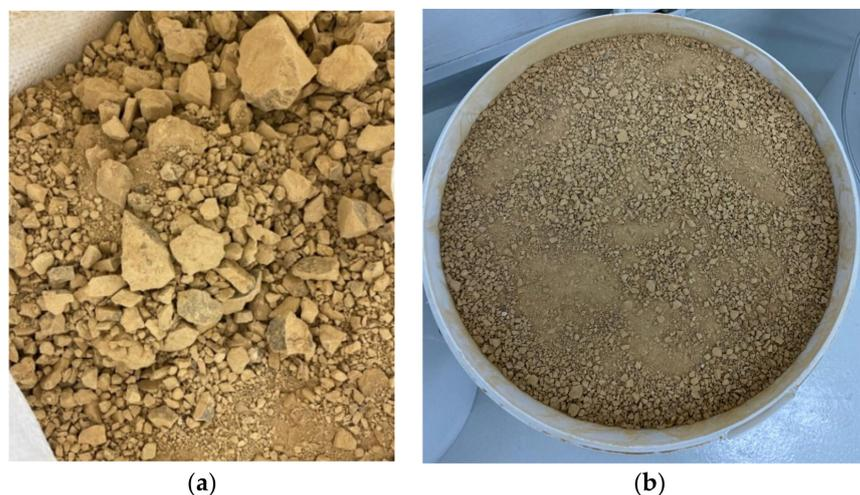
**Figure 1.** (a) natural soil sourced from land excavation; and (b) grinded natural soil.
