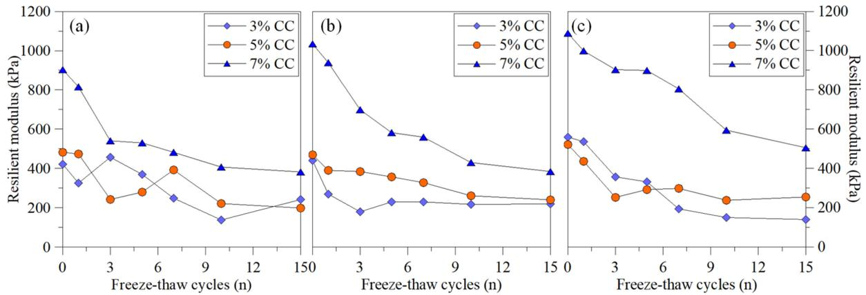
Figure 10. Resilient Modulus: (a) 3-day curing; (b) 7-day curing; and (c) 14-day curing.
