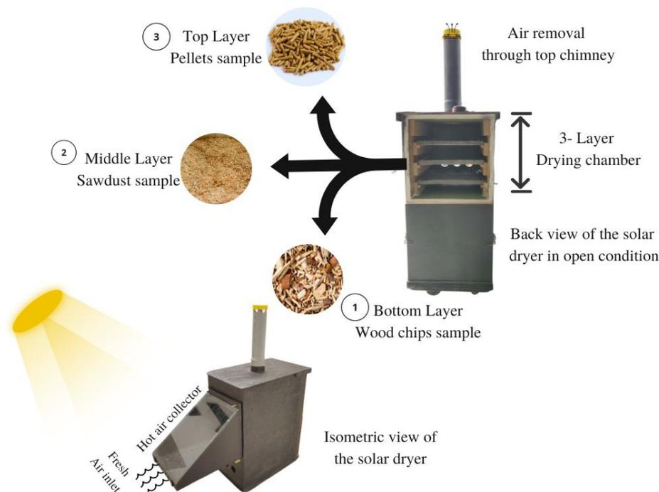
Figure 2. Experimental setup of the solar dryer for the investigations.
