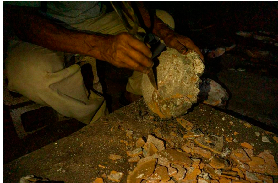
Figure 3. Black salt production; the mold is being broken to take the salt out. RAICES NGO (2023).
