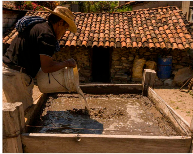
Figure 9. Distillation process. Hot water from the springs is being poured over the soil impregnated with salt. RAICES NGO (2023).
