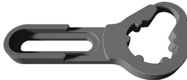
**Figure 2.** Three-dimensional data model of the used torque arm to upgrade a classic bicycle to an e-bike.
