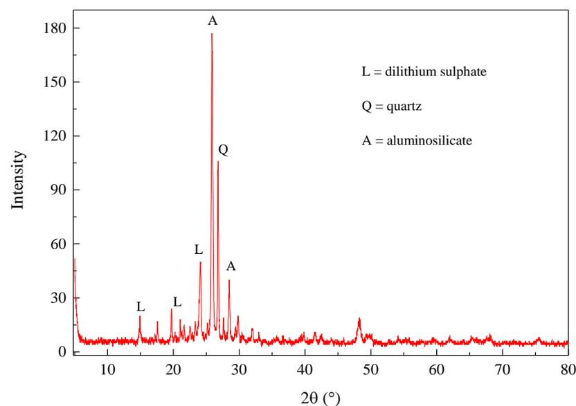
**Figure 1.** XRD patterns of LS used in the experiments.
