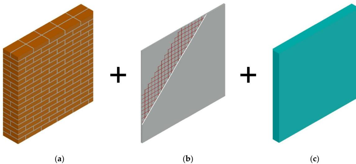
**Figure 4.** Conceptual scheme of integrated retrofit by means of composite materials: (a) existing envelope (brick masonry wall); (b) TRM system; and (c) thermal insulator (XPS).
