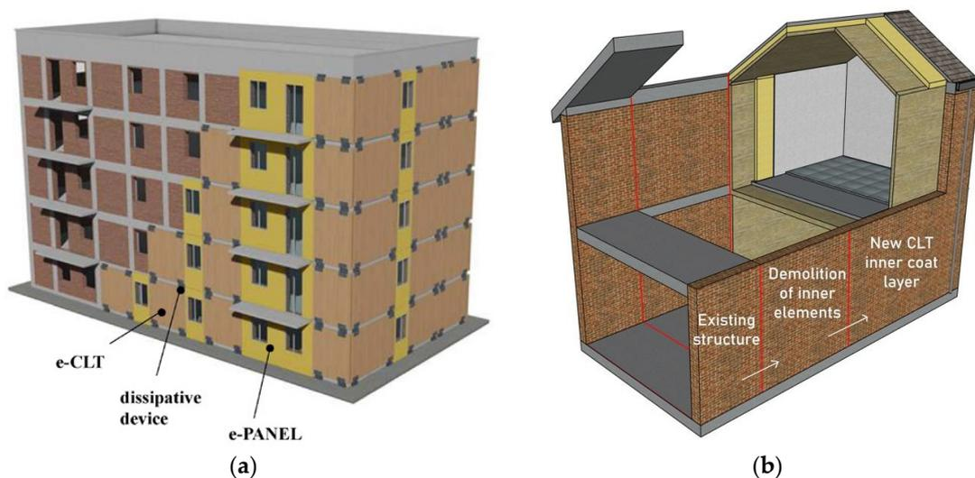
**Figure 3.** CLT panels for integrated retrofitting: (a) a conceptual representation of the solution proposed by Tardo and Margani [46]; (b) a schematization of work phases according to the “nested building” approach [48].
