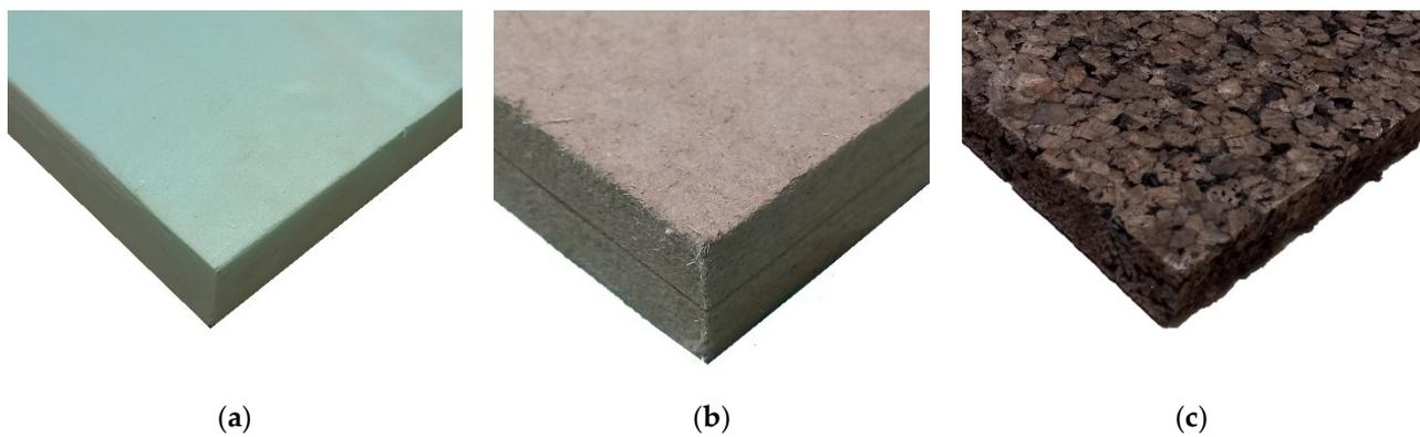
**Figure 6.** Thermal insulators: (a) extruded polystyrene (XPS); (b) wood fibreboard; and (c) expanded cork panel.
