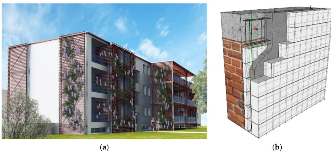
**Figure 2.** Integrated seismic and energy retrofit: (a) combination of structural, energy and architectural renovation using steel exoskeletons [37]; (b) visual representation of RC shell external structure for integrated refurbishment proposed in [41].
