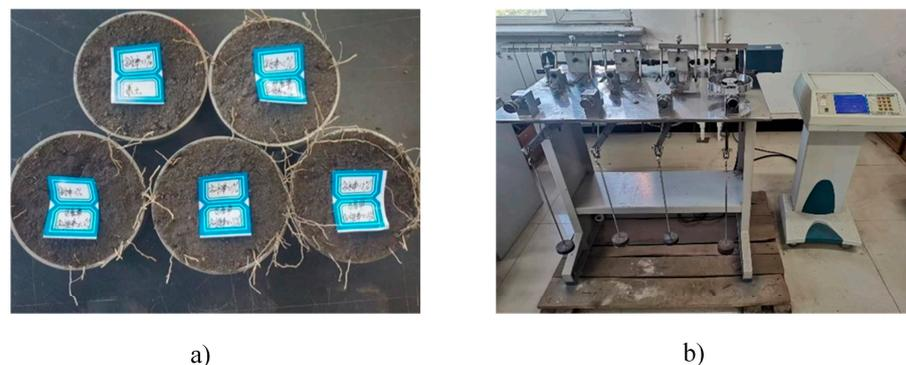
**Figure 3.** Straight shear specimens and equipment: (a) root-bearing soil ring cutter sample; (b) STSJ-5A intelligent electric instrument with four straight shears.
