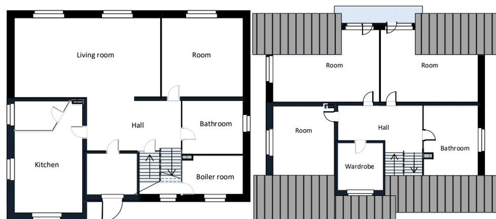
Figure 2. Ground floor and attic floor plans.
