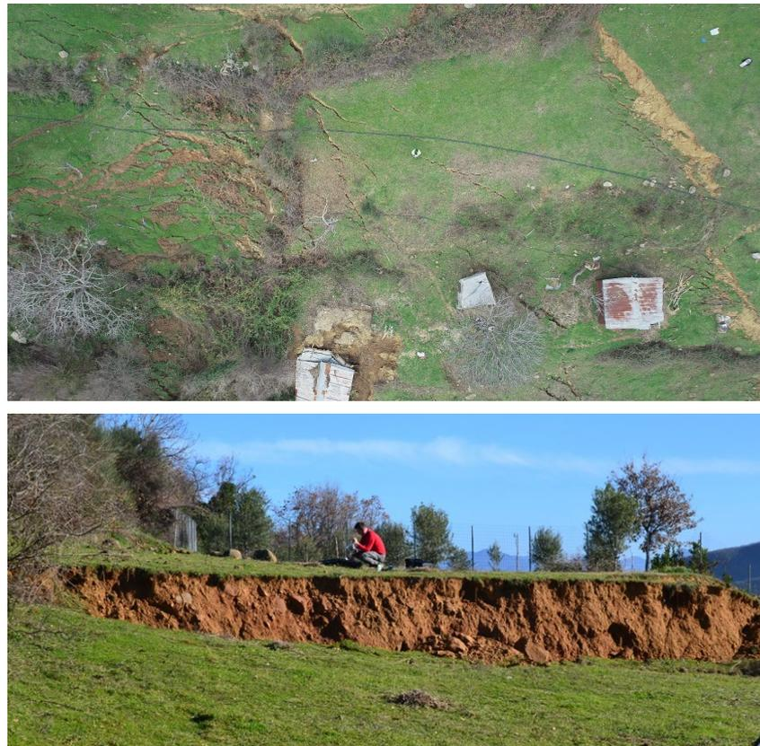
**Figure 2.** Fieldwork on 8 February 2021 in Ano Kerassovo village. (**Upper**): A characteristic UAV photo. Cracks are easily detected. The red arrow illustrates one large crack upward from the main road with a depth of almost one meter. (**Bottom**): The same crack as captured from a ground-based perspective.
