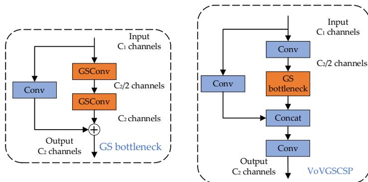
Figure 7. GS bottleneck and VoV-GSCSP network structure.
