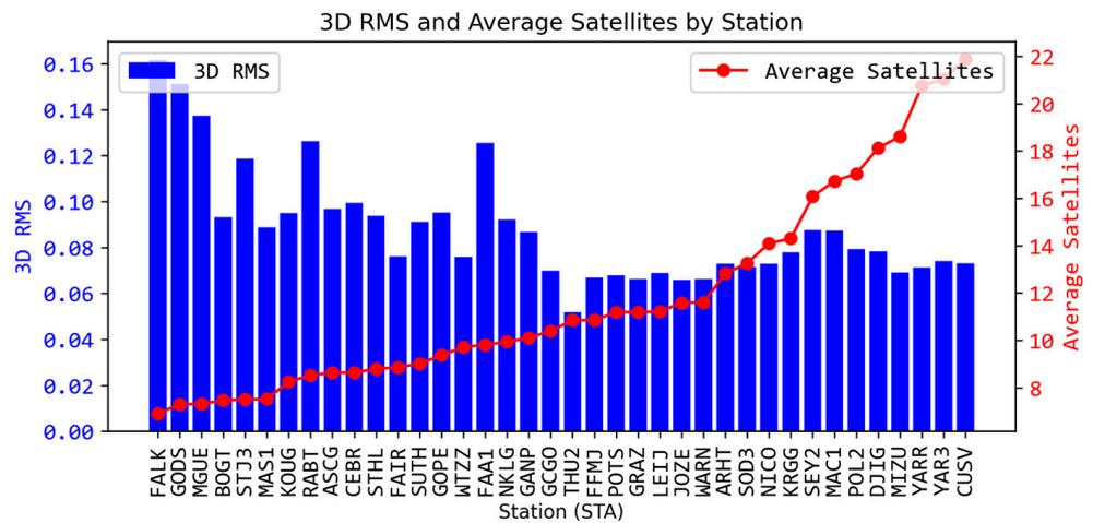
Figure 4. Average 3D RMS for each station as well as the number of visible satellites.
