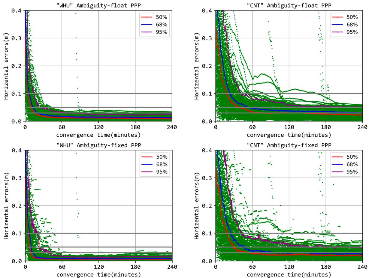
**Figure 15.** The positioning errors (green) alongside their 50% (red), 68% (blue), 95% (purple) quantiles for ambiguity-float (**top**) and ambiguity-fixed (**bottom**) “GEC”-combined PPP using the “WHU” and “CNT” products.
