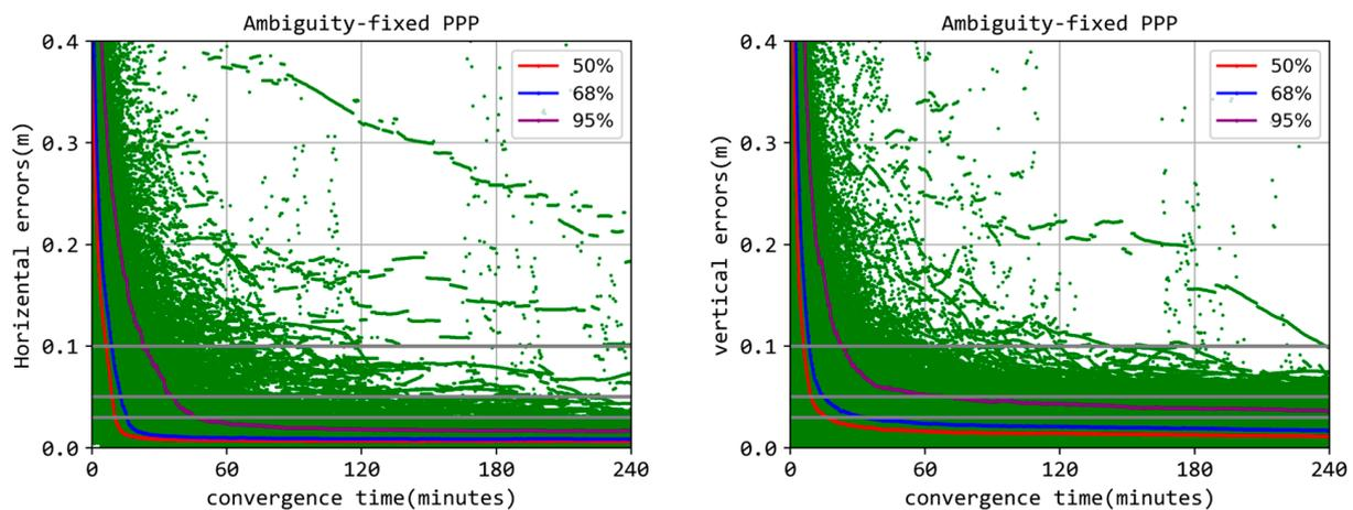
**Figure 14.** The positioning errors (green) alongside their 50% (red), 68% (blue), 95% (purple) quantiles for the horizontal (left) and vertical (right) components from ambiguity-fixed “GE” PPP with “WHU” products.
