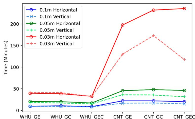
**Figure 12.** The convergence time of the horizontal and vertical positioning errors for ambiguity-float PPP to different thresholds by different processing combinations.
