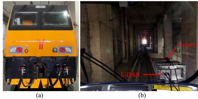
**Figure 9.** Experimental platform. (a) Train. (b) Install position of sensors.
