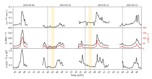
**Figure 3.** Time series of (top) RCS measured with Colibri (from ground to 150 m). In situ time series of  $\sigma_{abs}$  are presented in red and  $\alpha_{in-situ}$  in black (middle), and the bottom shows the total aerosol concentration. The highlighted regions indicate the calibration time frames.
