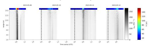
**Figure 5.** The binary color map of the  $\alpha_{Colibri}$  retrieved using the time series of the lidar ratio found in this study as input is shown for the whole campaign. At the top of the figure, the lidar ratio time series is labeled in the color map, and each date is separated by dashed vertical lines.
