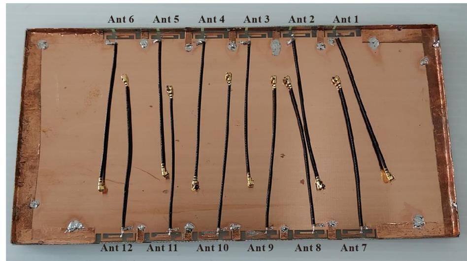
**Figure 8.** Fabricated MIMO twelve-antenna system.
