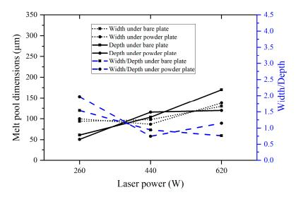
**Figure 7.** Melt pool width, depth, and width/depth measured from the printed single-track samples under the same laser speed (1.47 m/s).
