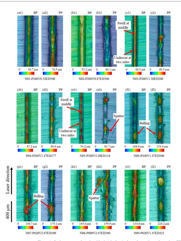
**Figure 3.** Surface topography colored by height for single-track samples on bare plate (BP) and powder plate (PP) with different laser powers and speeds. **(a1,a2)** P = 260 W, V = 0.52 m/s; **(b1,b2)** P = 260 W, V = 0.87 m/s; **(c1,c2)** P = 260W, V = 1.30m/s; **(d1,d2)** P = 260 W, V = 1.47 m/s; **(e1,e2)** P = 260 W, V = 2.20 m/s; **(f1,f2)** P = 440 W, V = 1.47 m/s; **(g1,g2)** P = 620 W, V = 2.07 m/s; **(h1,h2)** P = 800 W, V = 2.67 m/s; **(i1,i2)** P = 620 W, V = 1.47 m/s.
