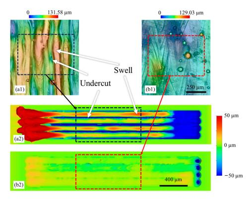
**Figure 11.** Surface topography of cube samples and multiple-track simulation, (**a1**) experiment and (**a2**) simulation for the high laser power and speed condition (440 W and 1.47 m/s); (**b1**) experiment and (**b2**) simulation for the low laser power and speed condition (260 W and 0.52 m/s).
