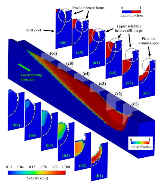
**Figure 10.** Melt pool swell-undercut formation with laser power 440 W and speed 1.47 m/s, (**a1–a6**), liquid fraction, (**b1–b6**), velocity, (**c1–c6**), location of cross sections.
