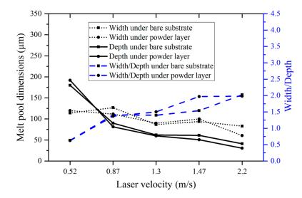
**Figure 5.** Melt pool width, depth, and width-to-depth measured from the printed single-track samples under the same power (260 W).
