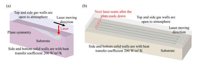
Figure 1. Boundary conditions: (a) single-track, (b) multiple-track.
