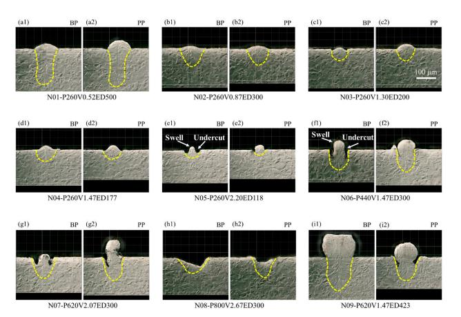
**Figure 4.** Cross-sectional view of melt pool morphology on bare plate (BP) and powder plate (PP) with different laser powers and speeds. (**a1,a2**) P = 260 W, V = 0.52 m/s; (**b1,b2**) P = 260 W, V = 0.87 m/s; (**c1,c2**) P = 260W, V = 1.30m/s; (**d1,d2**) P = 260 W, V = 1.47 m/s; (**e1,e2**) P = 260 W, V = 2.20 m/s; (**f1,f2**) P = 440 W, V = 1.47 m/s; (**g1,g2**) P = 620 W, V = 2.07 m/s; (**h1,h2**) P = 800 W, V = 2.67 m/s; (**i1,i2**) P = 620 W, V = 1.47 m/s.
