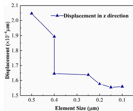
**Figure 4.** Mesh independence test by refining the mesh for the 1/4 RVE model.
