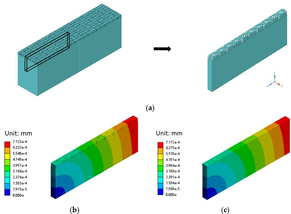
**Figure 6.** (a) Detailed model in the numerical validation; (b) Deformation of the detailed model; (c) Deformation of the homogenized model.
