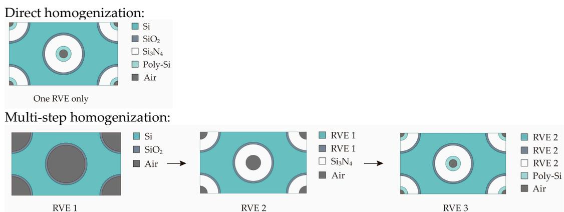
**Figure 5.** Schematic of two homogenization methods.
