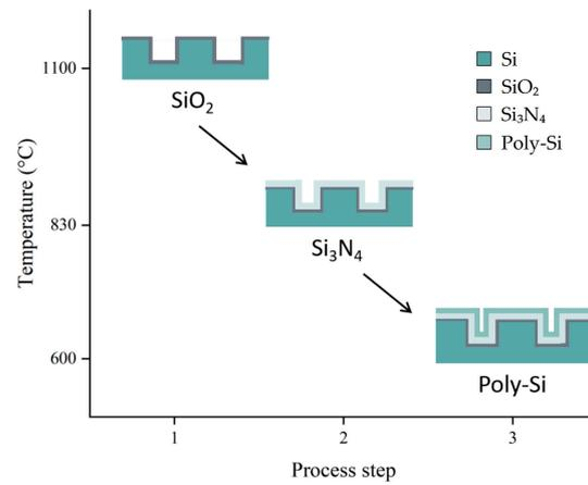
**Figure 1.** Simplified schematic of manufacturing process. Si substrate; SiO<sub>2</sub> layer deposition at 1100 °C; Si<sub>3</sub>N<sub>4</sub> layer deposition at 830 °C; Poly-Si layer deposition at 600 °C.
