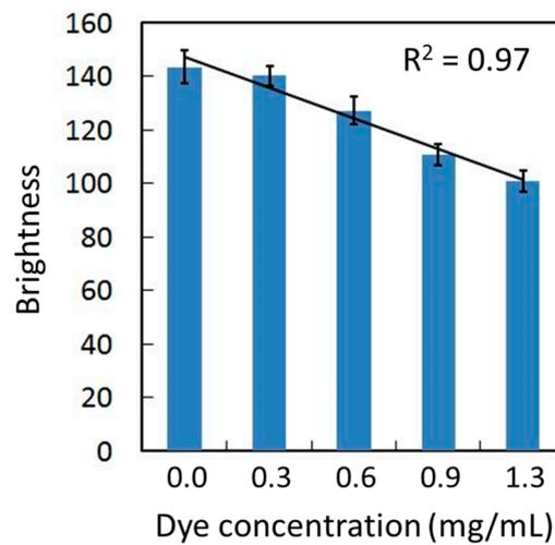
**Figure S1.** Calibration between dye concentration and brightness. The brightness of the colored water using the dye is linear in the range of our usage. The R-squared value is 0.97 when the data is linearly fitted.
