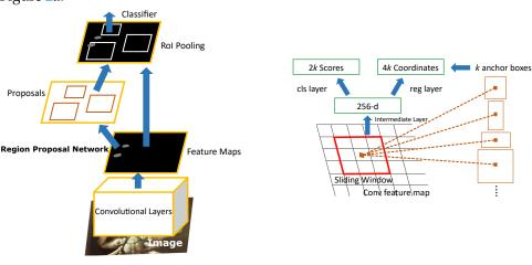
(a) Single, unified, end-to-end network(b) Region proposal network (RPN)Figure 2. Faster R-CNN with RPN [16].
