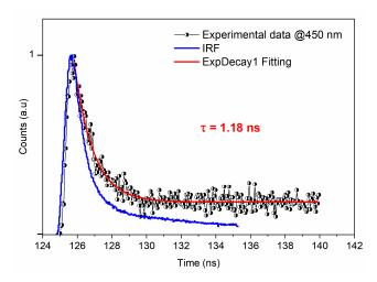
**Figure 7.** PL lifetime profile of  $(C_6H_{10}N_2)_4[CdBr_6][CdBr_4]_2$  at  $\lambda_{exc} = 375$  nm.
