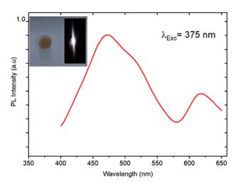
**Figure 6.** Emission spectrum for  $(C_6H_{10}N_2)_4[CdBr_6][CdBr_4]_2$  excited at 375 nm (inset: digital photo of the compound before and during excitation).
