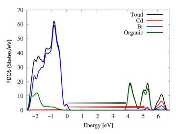
**Figure 9.** DOS of the  $(C_6H_{10}N_2)_4[CdBr_6][CdBr_4]_2$ . The separated PDOS contributions for each species are reported in different colors.
