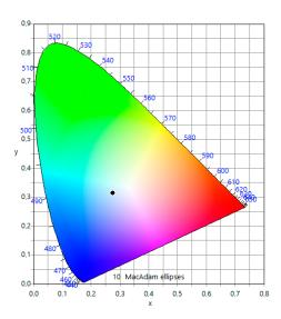
**Figure 8.** Color coordinates of the emitted white light in the CIE diagram (1931);  $\lambda_{exc} = 375$  nm.
