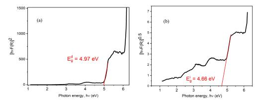
Figure 5. Tauc plot for (a) direct and (b) indirect gap calculation.
