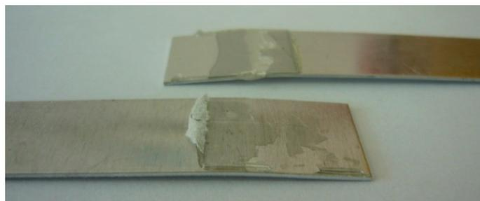
**Figure 4.** View of adhesive joints after strength test—the view of SCF—special cohesion failure.
