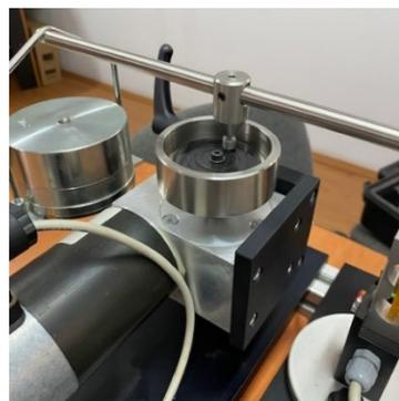
**Figure 8.** Pin on disk tribometer.
