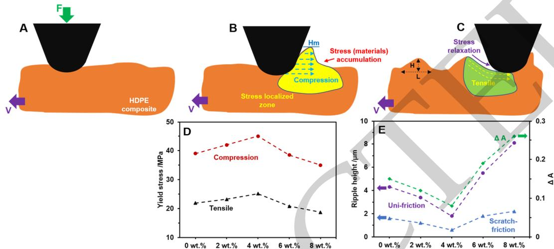
**Figure 9.** (A–C) graphically represent ripple deformation during the single-asperity scratch test; (D,E) show the relationships between the addition of  $\text{Si}_3\text{N}_4$  and the intrinsic mechanical properties, the ripple, and COF responses.
