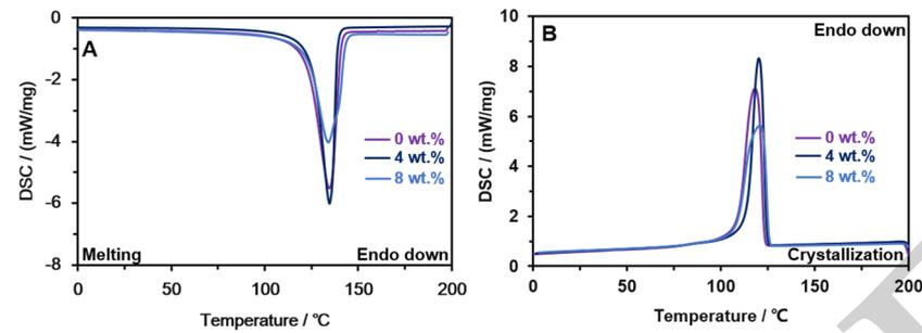
**Figure 4.** DSC results of the HDPE composites with a rate of 10 °C/min: (A) melting curves and (B) cooling (crystallization) curves.
