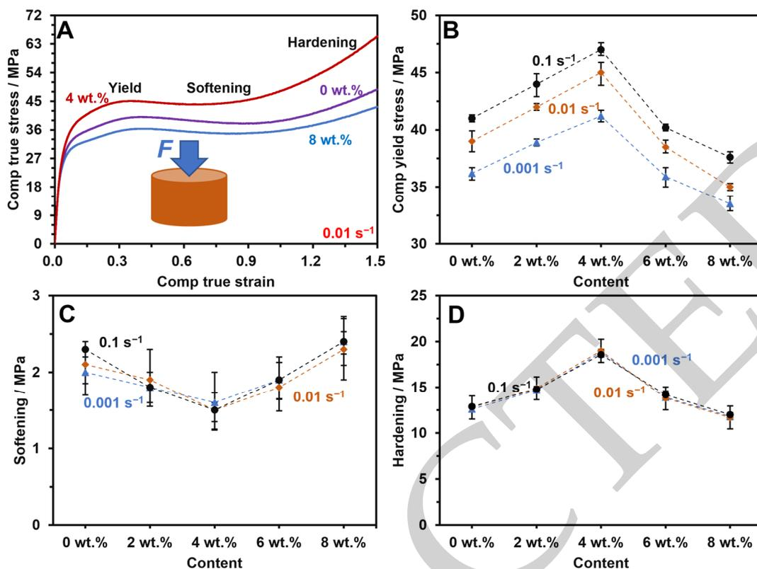
**Figure 3.** True strain-stress from the compression test of the HDPE composite: (A) complete strain-stress curve; (B) true yield stress, (C) strain-softening, and (D) strain-hardening, under different Si<sub>3</sub>N<sub>4</sub> contents and strain rates.
