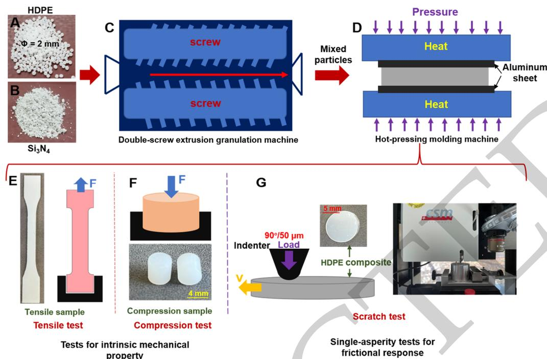
**Figure 1.** Sample preparation and testing apparatus: (A) HDPE granules; (B) silicon nitride powder ( $\text{Si}_3\text{N}_4$ ); (C) double-screw extrusion granulation for mixed particles; (D) hot-pressing molding machine for testing the samples. Tensile (E) and compression (F) tests for the intrinsic mechanical property. (G) Frictional response from the single-asperity scratching test.
