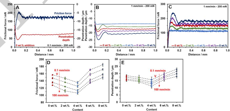
**Figure 5.** Frictional responses of the HDPE composites with different  $\text{Si}_3\text{N}_4$  contents: (A) penetration depth and corresponding frictional force; (B) penetration depth and (C) frictional force with increasing applied loads; (D) averaged frictional force and (E) penetration depth under different scratching velocities.
