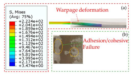
Figure 11. Joint failure diagram. (a) Simulation; (b) experiment.
