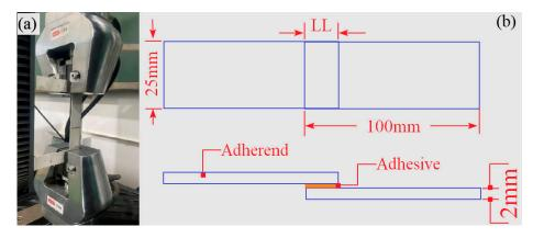
**Figure 6.** Specimen geometry size and tensile shear test device. (**a**) Tensile shear test device; (**b**) specimen geometry size.
