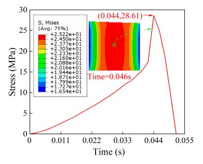
Figure 13. The stress from the center region element.
