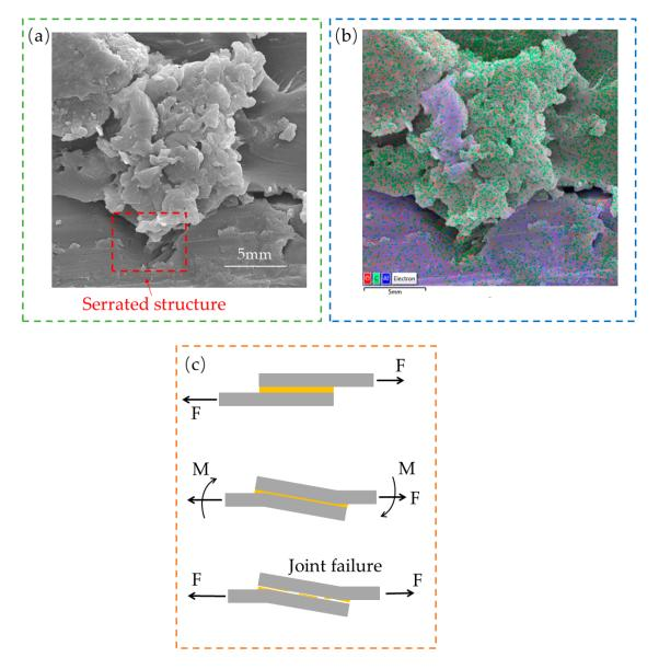
**Figure 19.** Schematic diagram of interfacial bonding and bending moment. (**a**) Interfacial bonding; (**b**) EDS analysis; (**c**) bending moment.
