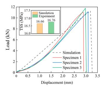
Figure 22. The verification of ML prediction results.
