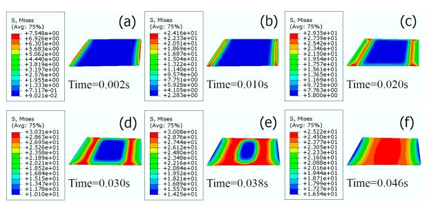
element at 0.046 s (seen in Figure 13), and it was discovered that the maximum stress was 28.61 MPa at 0.044 s.
