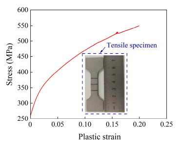
Figure 5. Real strain-stress curve of 2A12-T4 aluminum alloy.
