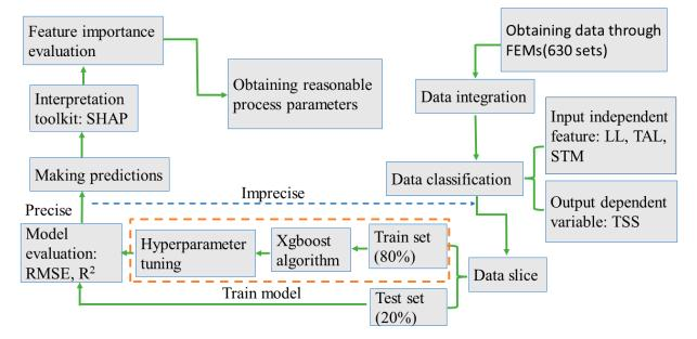
**Figure 15.** The flow chart for predicting the metal–metal bonding performance based on the Xgboost ML algorithm.
