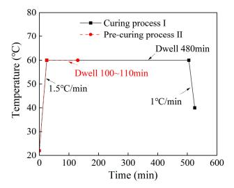
Figure 2. Curing process of DW-3 adhesive.
