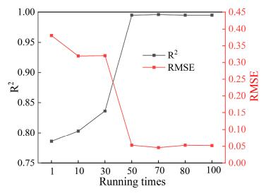
Figure 16. The change graphs of RMSE and R<sup>2</sup> values with the running times of the Xgboost model.
