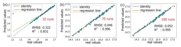
Figure 17. Comparison of predicted TSS and true TSS values: (a) 10 runs; (b) 70 runs; (c) 100 runs.
