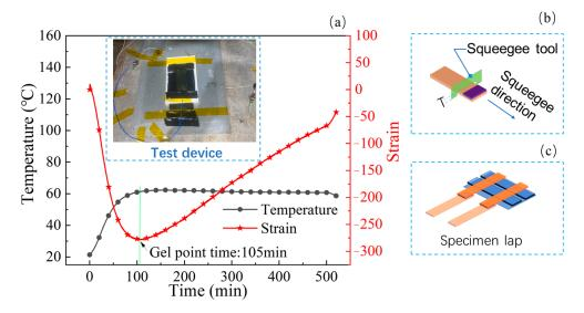
**Figure 3.** The diagram of the GP acquisition device, squeegee tool, and specimen lap. (a) GP acquisition device; (b) squeegee tool; (c) specimen lap.
