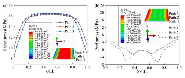
Figure 14. Stress distribution along three paths. (a) Shear stress; (b) peel stress.
