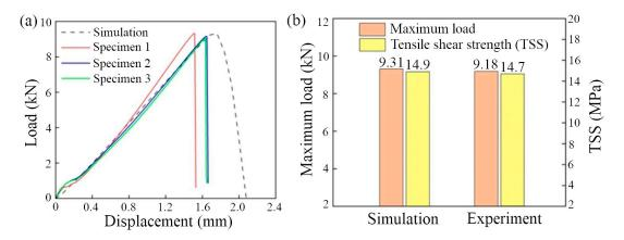
**Figure 9.** The results for the experiment and simulation of SLJs. (a) Load–displacement curves; (b) comparison of the maximum load and TSS values.
