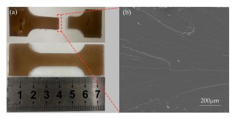
Figure 10. The tensile specimen fracture diagram of the adhesive: (a) macro; (b) micro.
