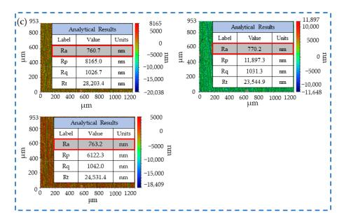
Figure 1. Metal surface roughness values: (a) Type-1; (b) Type-2; (c) Type-3.
