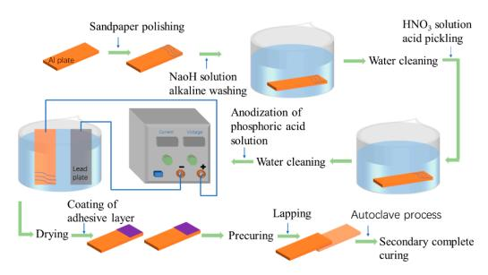
Figure 4. The whole process of the bonding experiment.
