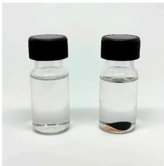
Figure S4. The longevity verification experiment in a 1 M LiPF 6 electrolyte with/without the prepared electrode after 60 days
