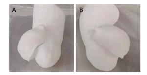
**Figure 7.** Additive manufacturing of a TPU 0.3 mm thick bicuspid aortic valve using an additional reinforcement scan layer using a laser power of 12 W (preset TPU-1). Double contour (**A**) and edge (**B**) enable successful manufacturing.
