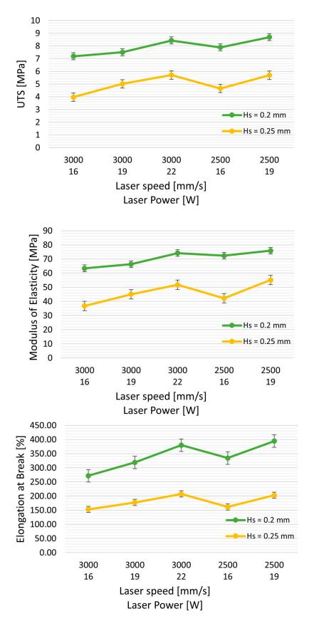
**Figure 4.** Effect of Hs (hatching distance) on mechanical properties: UTS (ultimate tensile strength), elongation at break, and modulus of elasticity. Green curves represent the properties with Hs = 0.20 mm, and yellow curves represent Hs = 0.25 mm, with varying laser powers and at two speeds, 3000 and 2500 mm/s.
