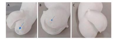
**Figure 6.** Model of an aortic valve with a simple contour. (**A**) A 0.3 mm thickness valve using a low-energy technique (preset TPU-2 with  $\text{Ed} = 0.21 \text{ J/mm}^3$ ) and (**B**) a 0.4 mm thickness valve both exhibit small holes (indicated by the blue arrow) in the thin printed section. In comparison (**C**), the 0.5 mm thickness TPU model is flawless.
