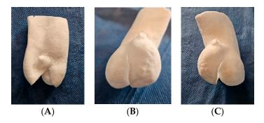
**Figure 8.** Additive manufacturing of bicuspid valve TPE models with thicknesses of (**A**) 0.5 mm, (**B**) 0.8 mm, and (**C**) 1.3 mm, obtained with the TPE-7 preset of 14 W and laser speed of 30,000 dps (1800 mm/s). (**A**) A 0.5 mm thick model: loss of shape memory with sagging. (**B**) A 0.8 mm thick model: flexible and resistant to handling. (**C**) A 1.3 mm thick model: retains adequate flexibility with greater strength.
