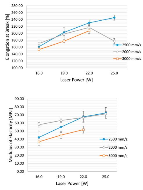
**Figure 3.** Effect of laser speed and power on mechanical properties: UTS (ultimate tensile strength), elongation at break, and modulus of elasticity. Hs (Hatching distance) is held constant at 0.25 mm, while the laser power varies from 16 W to 25 W and the speed from 3000 mm/s to 2000 mm/s.
