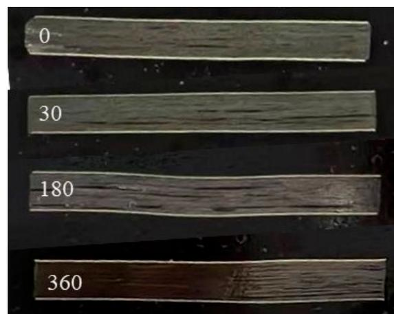
**Figure 8.** Interlayer cracks before and after hygrothermal accelerated aging.
