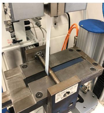
**Figure 5.** The test device according to VDI guideline 2019 with a clamped test specimen.
