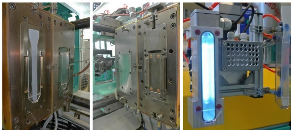
**Figure 2.** A pre-treatment module consisting of housing with vacuum suction cups for transferring the pre-molded part and an integrated UVC lamp (right) and a 2c injection molding tool for the production of TP/LSR composite test specimens with a fixed tool half (middle) and a movable tool half (left).
