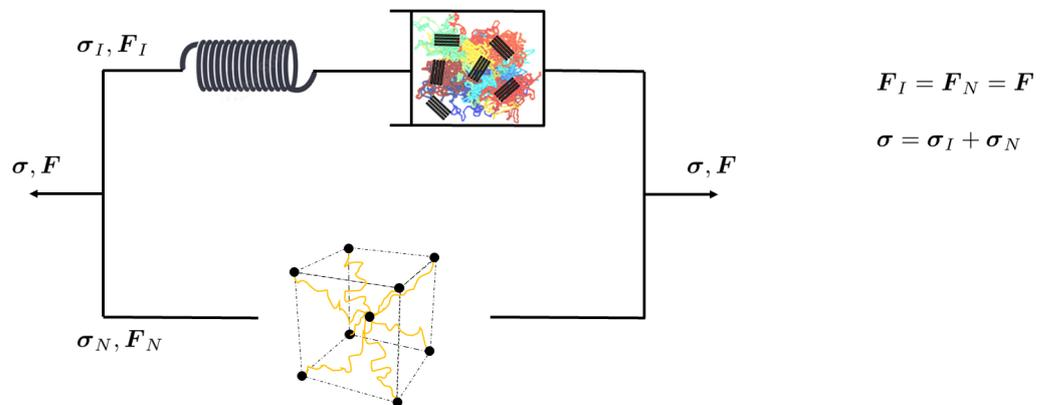
**Figure 4.** Schematic representation of intermolecular and network resistances in corresponding rheological model.
