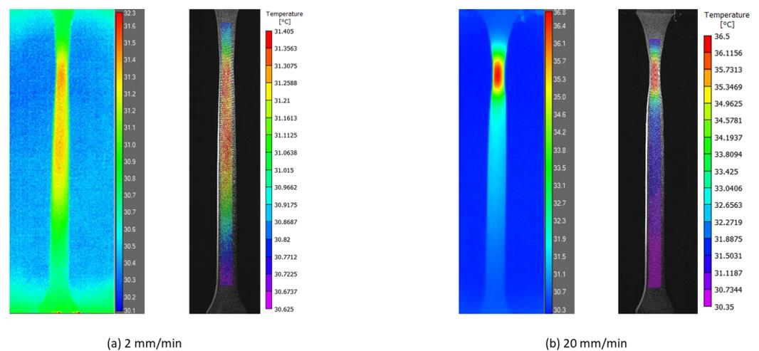
**Figure 2.** Temperature field mapping from IR camera recording to DIC post-processing of PP/HDPE blend at different loading speeds.
