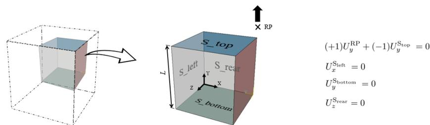
**Figure 5.** A one-eighth finite element (FE) model with corresponding boundary conditions.
