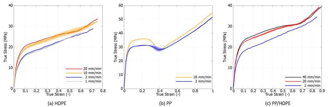
**Figure 7.** Experimental true stress–strain curves under tension at different strain rates at room temperature .
