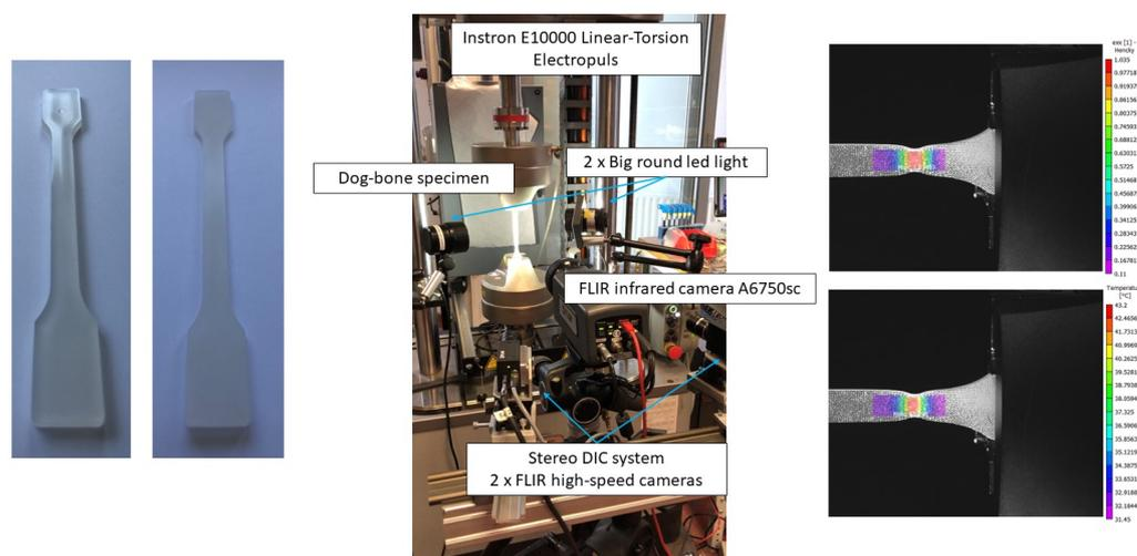
**Figure 1.** ISO-527 type-1A dog-bone specimen preparation (left), experimental setup (middle), and DIC measurements (right).
