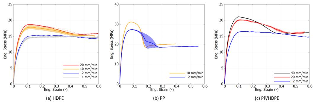
**Figure 6.** Experimental engineering stress–strain curves under tension at different strain rates at room temperature .
