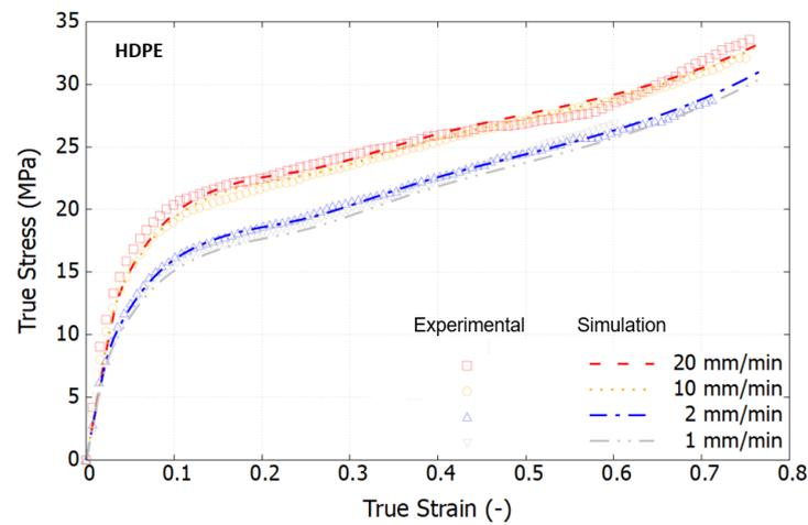
Figure 9. Comparison of the true stress–strain curves of HDPE between the model and the test at different loading speeds.
