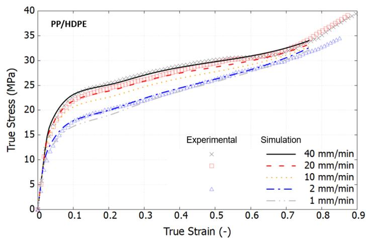
Figure 11. Comparison of the true stress–strain curves of the PP/HDPE blend between the model and the test at different loading speeds.
