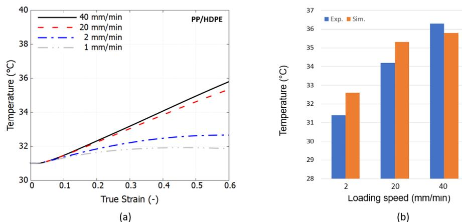
**Figure 12.** Temperature evolution: (a) prediction at different loading speeds using SE test and (b) comparison to experimental measured peak temperature at true strain of 60%.
