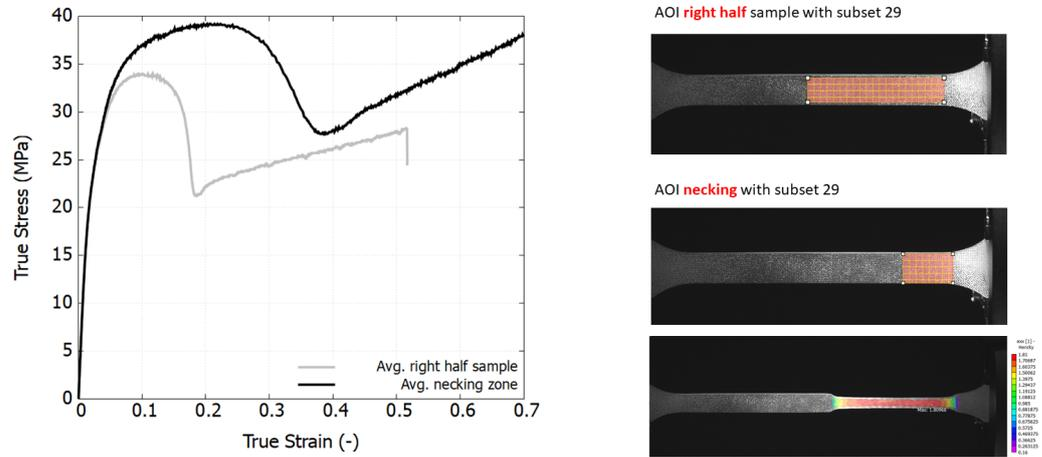
**Figure 3.** The effect of the Area of Interest (AOI) on true stress–strain response of a PP 576P specimen at a loading speed of 10 mm/min.
