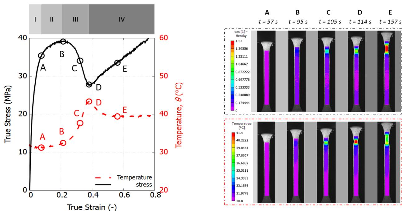
**Figure 8.** Experimental stress–strain response and temperature evolution of a PP 576P specimen under tension at 10 mm/min (left); local profile of strain and temperature fields (right).
