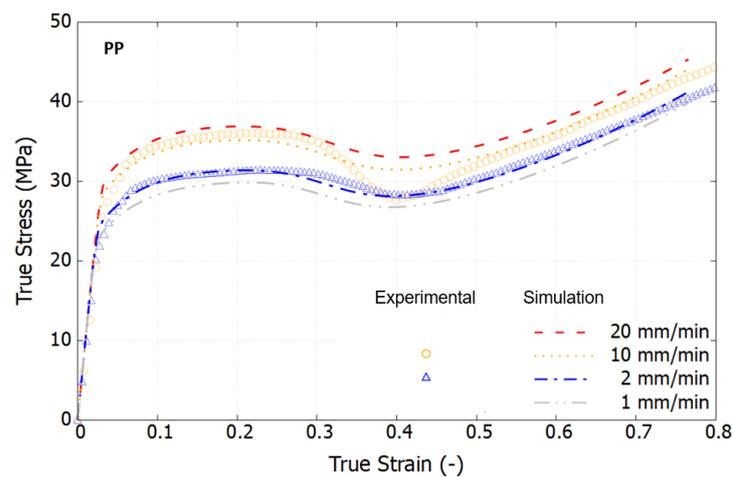
Figure 10. Comparison of the true stress–strain curves of PP between the model and the test at different loading speeds.
