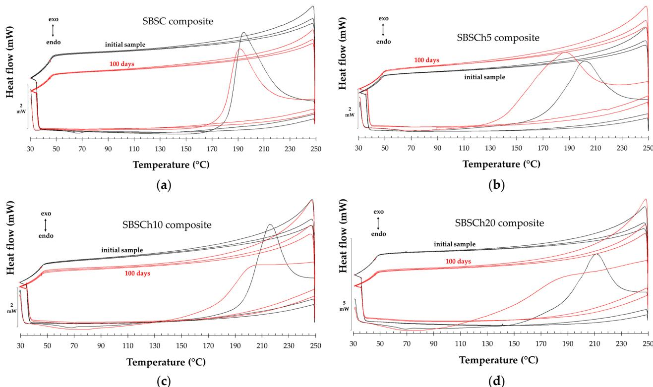
**Figure 12.** Comparative DSC thermograms of studied polymer composites without (a) and with incorporated *Chlorella vulgaris* biomass percentages of (b) 5%, (c) 10%, and (d) 20%, recorded on pristine samples (black lines), and on samples after 100 days of biodegradation (red lines), in dynamic thermal regime with 3 heating–cooling cycles, in the temperature range 30–300 °C, at a rate of 10 °C/min.
