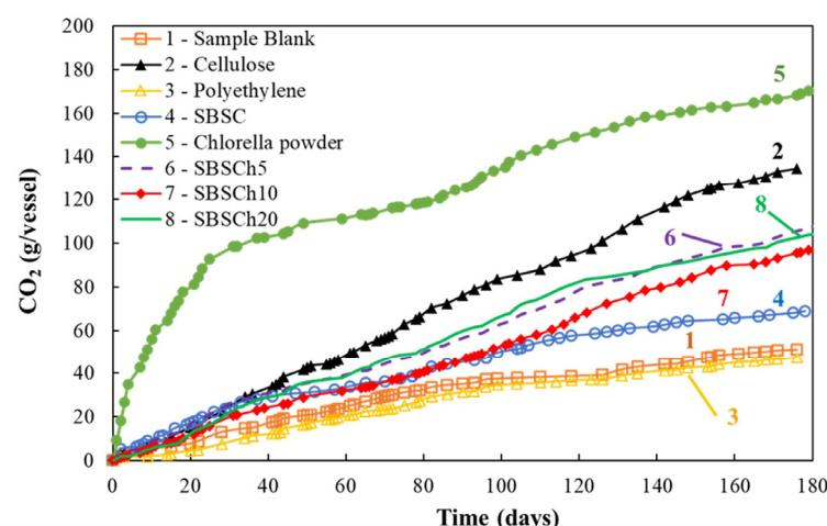
**Figure 2.** Evolution of  $\text{CO}_2$  mass (g/vessel) trapped in the  $0.5\text{ N}$  NaOH solution in the biodegradation test (industrial composting).
