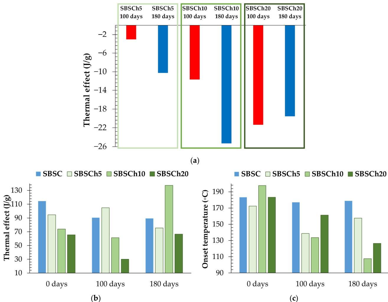
**Figure 13.** Representation of (a) normalized endothermal effect (J/g) registered in the 50–110 °C domain, (b) normalized exothermal effect (J/g), and (c) onset temperature variations in the exothermal effect, observed in the first cycle of heating for SBS composites filled with *Chlorella vulgaris* biomass.
