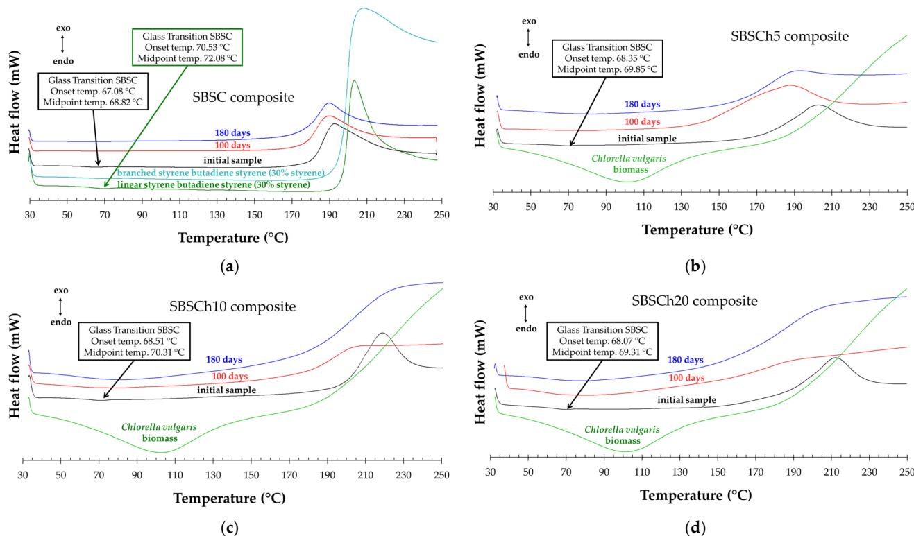
**Figure 11.** DSC curves of tested polymers recorded for samples heated from 0–300 °C at 10 K min<sup>−1</sup> heating rate: (a) SBSC composite before and after 100 and 180 days compared with the SBS used to prepare the polymer blends, (b) SBSCh5 and *Chlorella vulgaris* powder, (c) SBSCh10 and *Chlorella vulgaris* powder, (d) SBSCh10 and *Chlorella vulgaris* powder.
