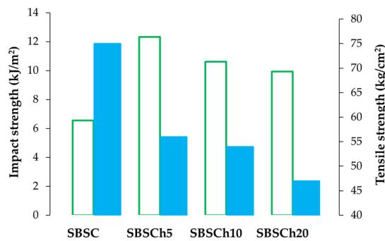
**Figure 4.** Compared values of impact strength (green empty bar) with tensile strength (blue bar) for SBS composites with different loaded microalgae biomass content.
