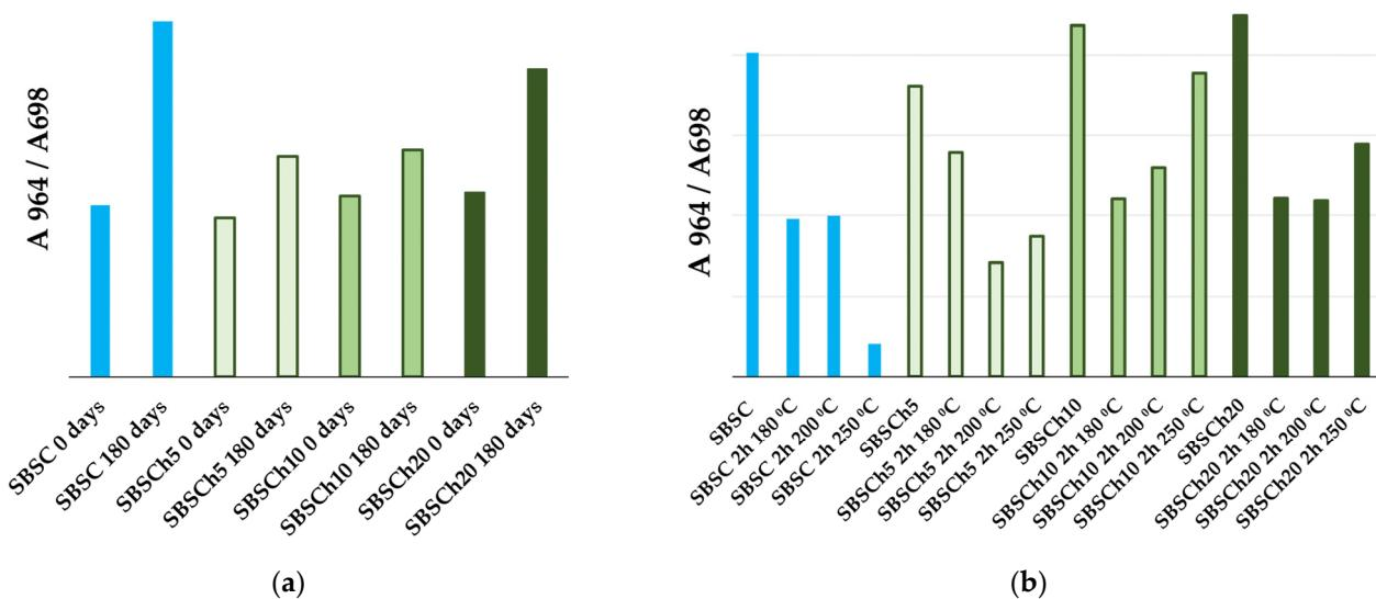
**Figure 8.** Comparison of absorbance ratios  $A_{964}\text{ cm}^{-1}/A_{698}\text{ cm}^{-1}$  calculated for initial samples (blue bars) that undergo (a) a biodegradation test, and, respectively, (b) a thermal degradation test (green bars).
