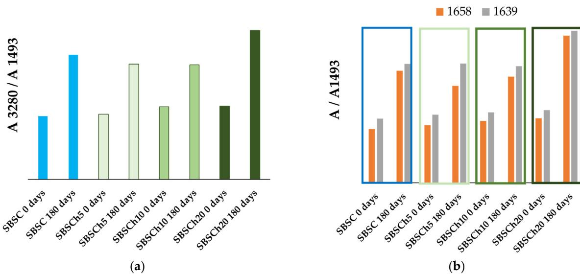
**Figure 9.** Compared values of absorbance ratios for studied samples before (blue bars—0 days) and after (green bars—180 days) the biodegradation test, calculated as absorbance values at  $3280\text{ cm}^{-1}$  (a), and respectively, at  $1658\text{ cm}^{-1}$  (orange bar) and  $1639\text{ cm}^{-1}$  (gray bar) (b), relative to absorbances measured at  $1493\text{ cm}^{-1}$ .
