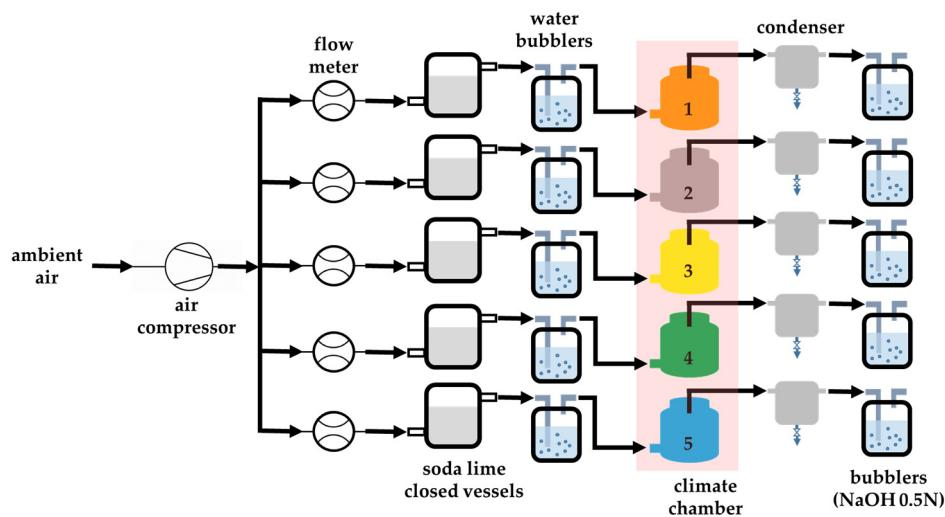
**Figure 1.** Schematic representation of the laboratory biodegradation testing installation.
