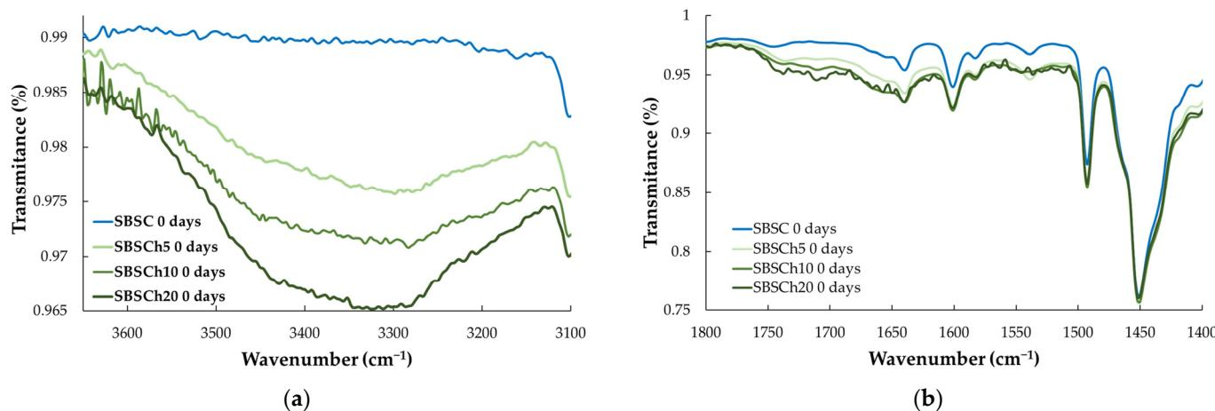
**Figure 7.** Infrared spectra of SBS-based composites before biodegradation in the region: (a) 3600–3100  $\text{cm}^{-1}$ , and (b) 1800–1400  $\text{cm}^{-1}$ .
