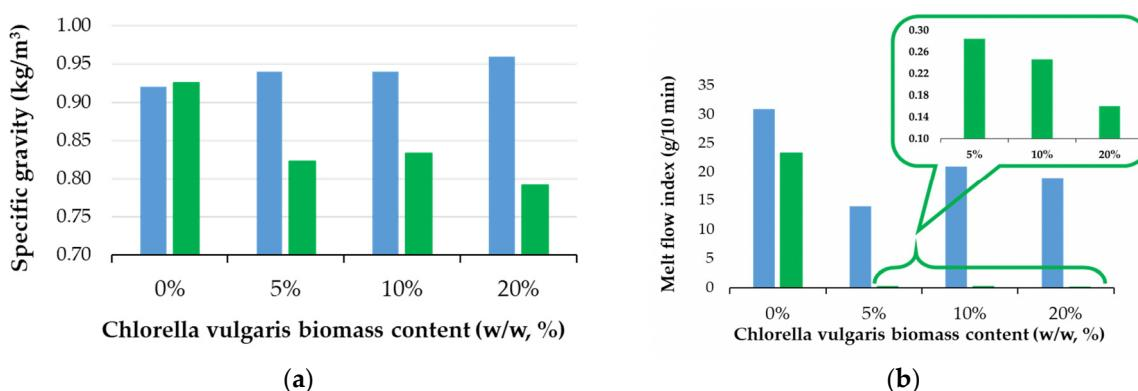
**Figure 5.** Physical properties of polymer composites: (a) specific gravity and (b) melt flow index for initial samples (blue bar) compared with samples after 180 days of an industrial composting biodegradation test (green bar).
