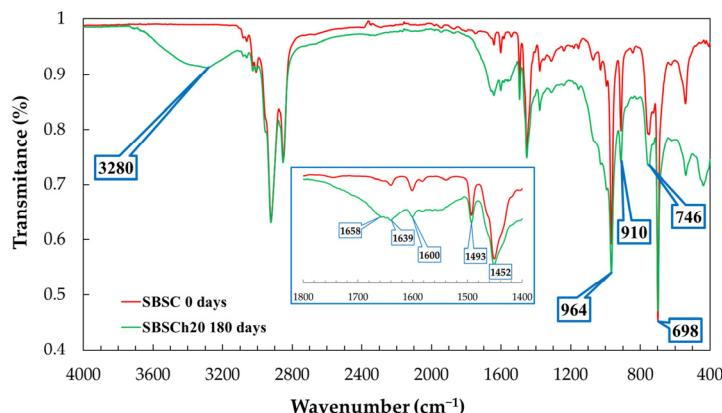
**Figure 6.** Infrared spectra of SBSC (initial, red line) compared with infrared spectra of SBSCh20 (after 180 days biodegradation test, green line).
