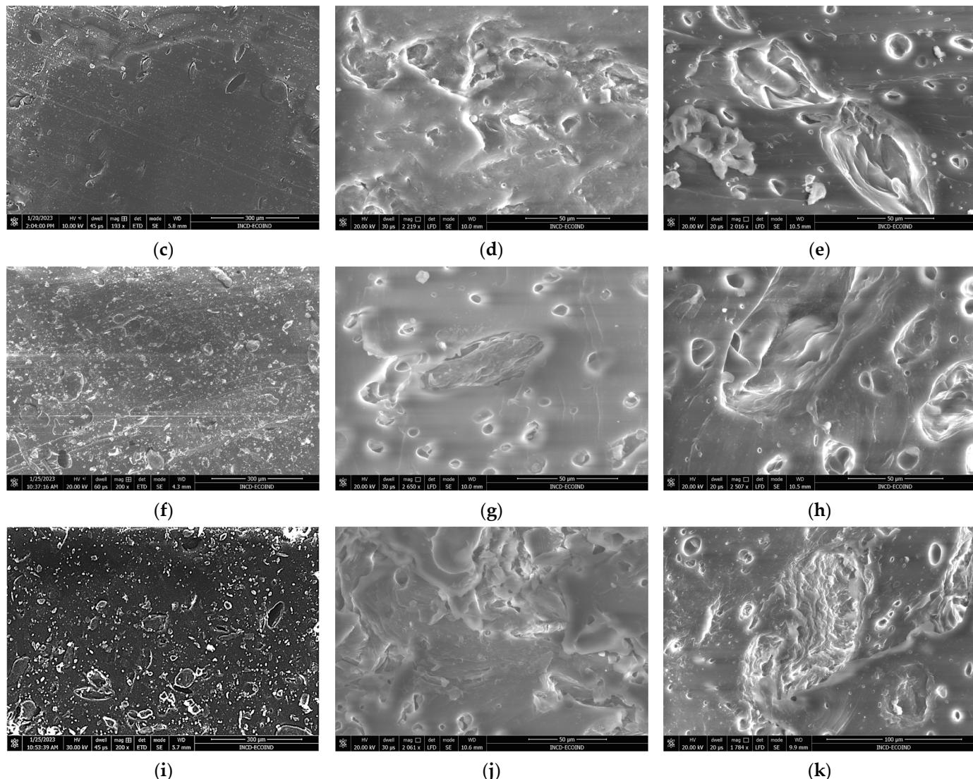
**Figure 10.** SEM images of polymer SBS composites, (a) SBSC initial sample, (b) SBSC after 180 days and SBS Chlorella composites, (c) SBSCh5 initial sample, (d) SBSCh5 after 100 days, (e) SBSCh5 after 180 days, (f) SBSCh10 initial sample, (g) SBSCh10 after 100 days, (h) SBSCh10 after 180 days, (i) SBSCh20 initial sample, (j) SBSCh20 after 100 days, and (k) SBSCh20 after 180 days.
