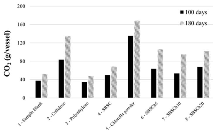
**Figure 3.** Comparative values of CO<sub>2</sub> mass (g/vessel) absorbed in the industrial composting biodegradation test: after 100 days, and 180 days.
