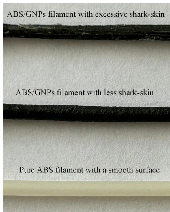
**Figure 4.** Surface images of the pure ABS and composite filaments.
